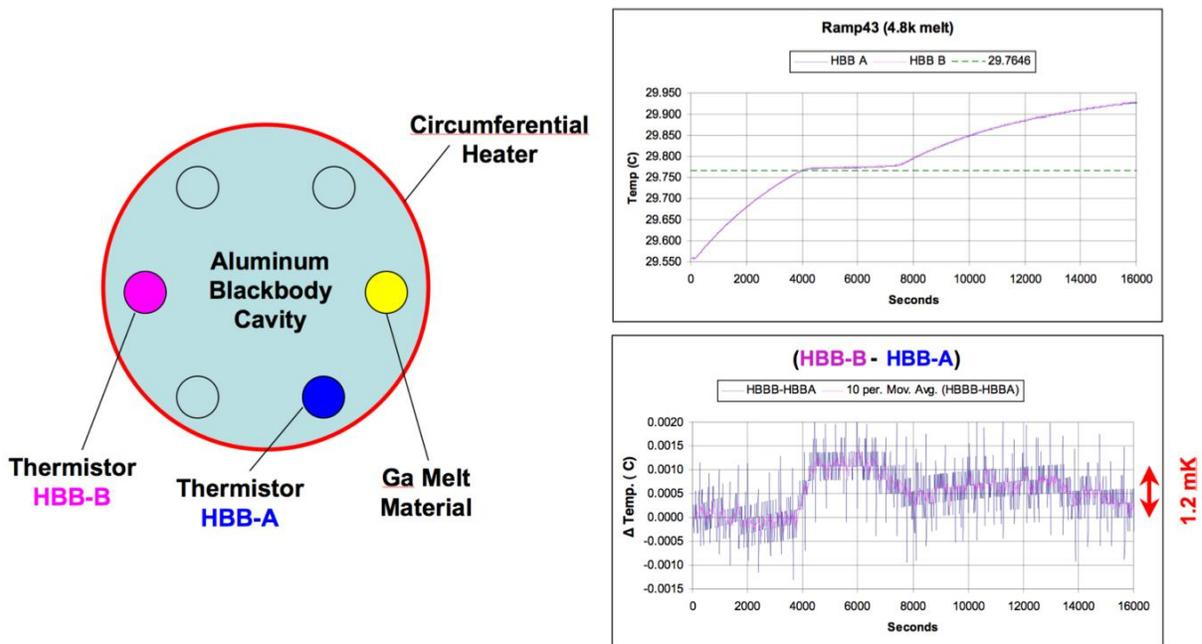
**Figure 9.** Gradients in the blackbody cavity during a “fast” 4,800 second melt are on the order of 1.2 mK. The lower right plot shows the temperature difference in the two thermistors located as shown in the figure on the left.
