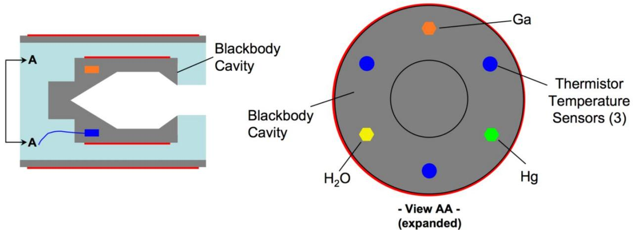
**Figure 10.** Implementation of the absolute temperature scheme requires integrating small quantities of different phase change materials into the aluminum blackbody cavity, interleaved between the thermistor temperature sensors to be calibrated. The view on the right is an expanded end view of the cavity only.
