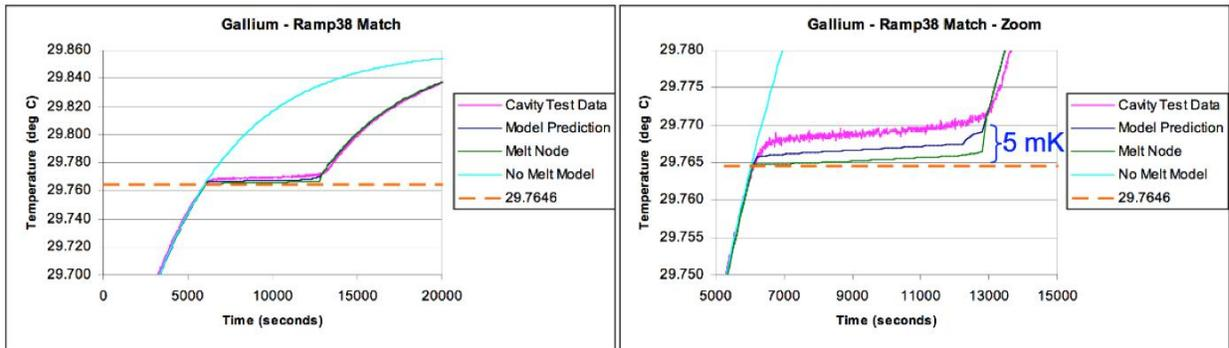
**Figure 4.** Typical gallium melt signature obtained with UW blackbody mock-up system. The plot on the right is an expanded view of the data potted on the left. The aqua colored rising exponential shows the temperature response of the blackbody cavity to constant power if no gallium were present. The plot on the right clearly shows that this melt event can be distinguished to within 5 mK.
