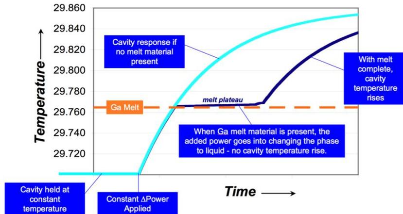
**Figure 5.** Sequence of events during a typical melt of gallium as configured in Figure 3. After initial stabilization in the constant temperature mode, a constant power is used to transition through the melt plateau.
