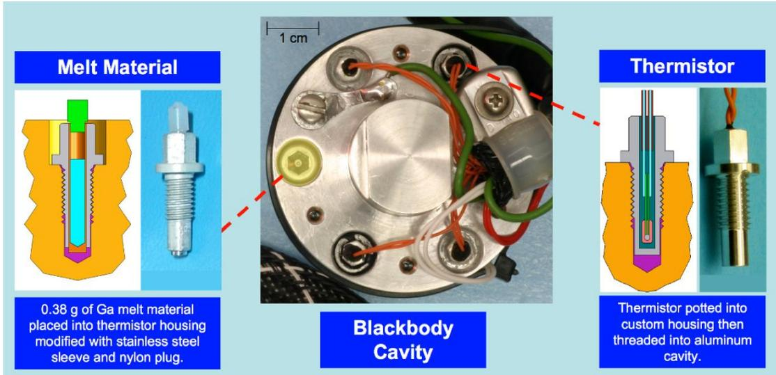
**Figure 3.** Configuration used to demonstrate the absolute temperature calibration concept, using a UW-SSEC mock-up blackbody. Small quantities (<1g) of different phase change materials are integrated into custom housings that have the same geometry as the temperature sensors. Threaded holes in the blackbody cavity accept either thermistors or one of the phase change materials (gallium is shown).
