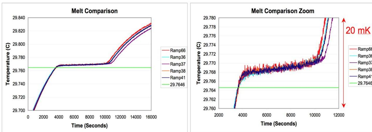
**Figure 6.** Repeatability of five different gallium melts is better than 2 mK. Melts spanned a 9-month period. The plot at right with a full scale of 20 mK is an expanded view of the data plotted at left.
