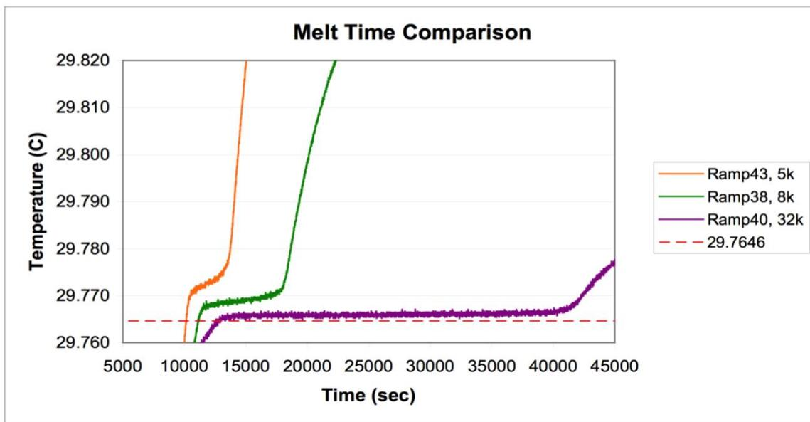
**Figure 7.** Gallium melts of different duration. The plateau temperatures of a melt more closely approaches the true gallium melt temperature for longer melt times.
