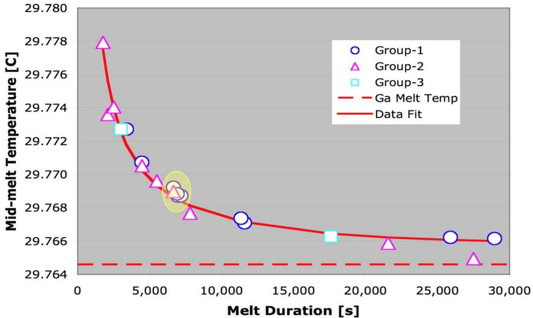
**Figure 8.** Gallium mid-melt temperature for 20 different melts of different durations. The data asymptotically approaches the true gallium melt temperature to within 1 mK at longer melt times.
