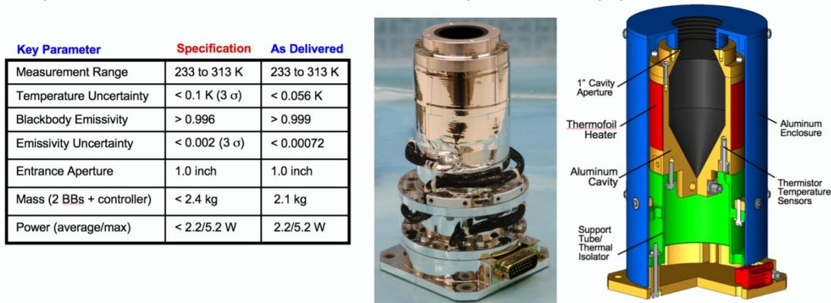
**Figure 1.** The GIFTS EDU blackbody top-level specifications and as-delivered performance are shown in table at left. A photo of the as-delivered hardware is shown in the middle without the enclosure. The cut-away figure on the right illustrates the key features of blackbody, including the thermistor locations and painted aluminum cavity.
