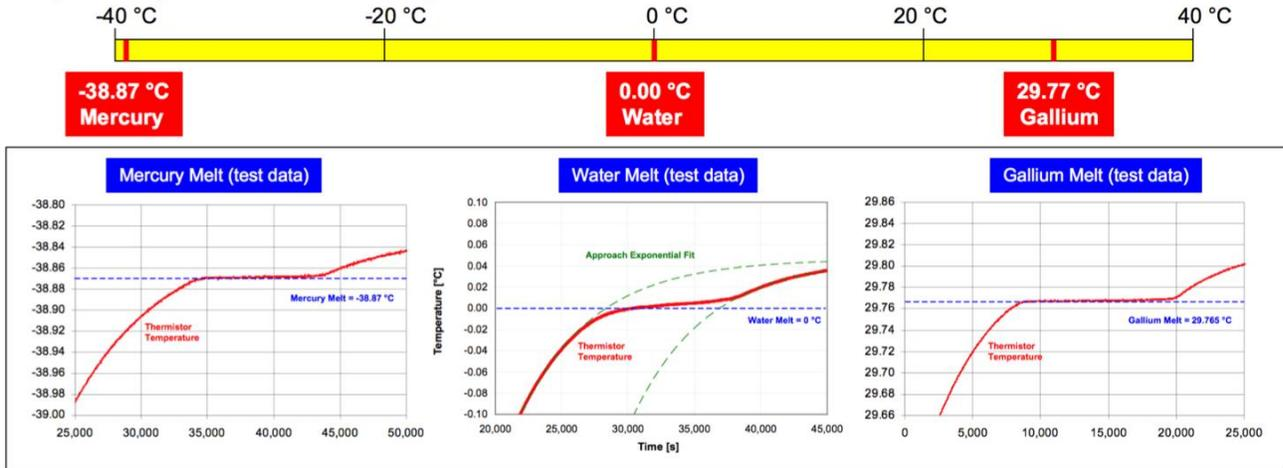
**Figure 11.** Melt signature test data for mercury, water, and gallium configured as illustrated in Figure 3 show that the melt plateau can be easily distinguished to within 10 mK. These three melts establish the thermistor calibration from -39 to 30 °C.
