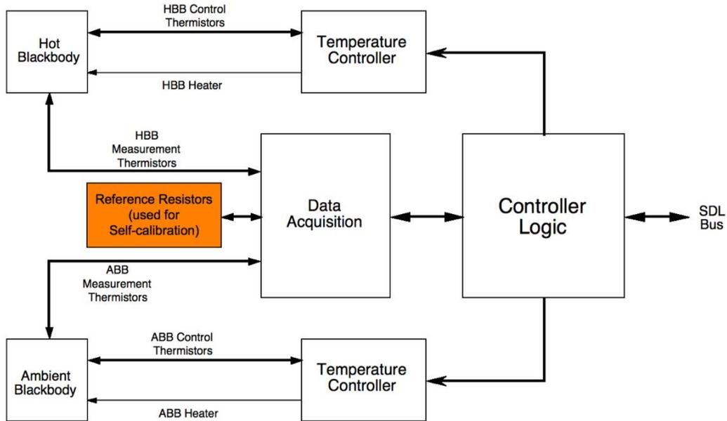
**Figure 2.** The blackbody controller provides independent temperature measurement and control for both blackbodies. At each data collection cycle the on-board reference resistors are measured along with the blackbody thermistor resistances – providing self-calibration.
