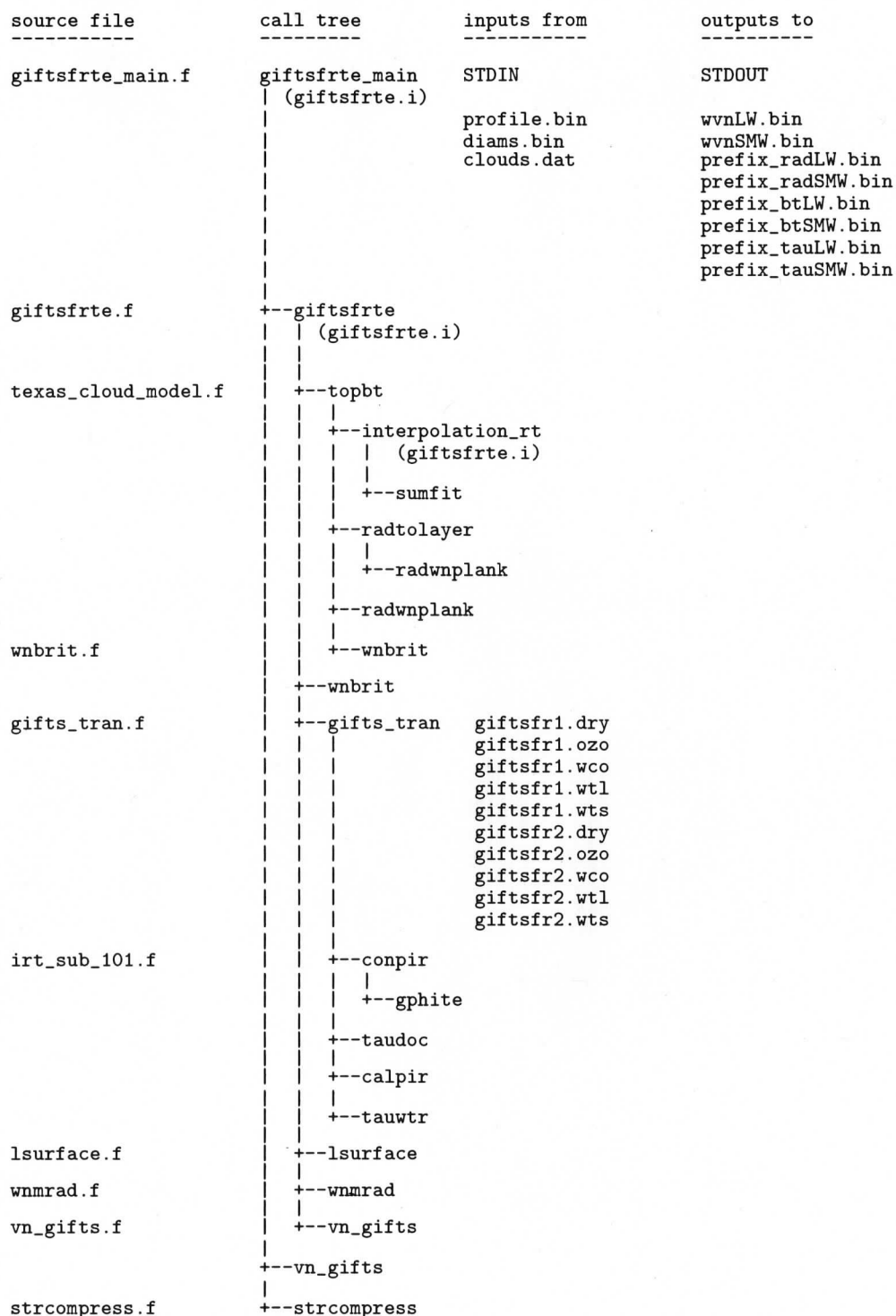
Figure 3: Call tree for upgraded GIFTS fast radiative transfer model (GIFTSFRTE). Inputs are from coefficient files, MM5 atmospheric profile files and from standard input, typically in the form of a redirected parameter file.
