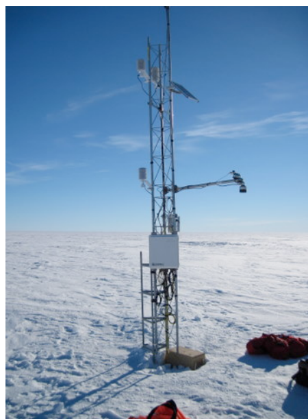
New AWS installed at Byrd AWS site on January 18 th , 2011
