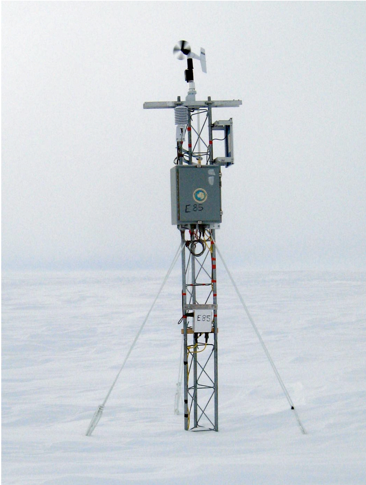
D85 AWS 8986 before being replaced with AWS 8912 (both AWS2B type AWS)
