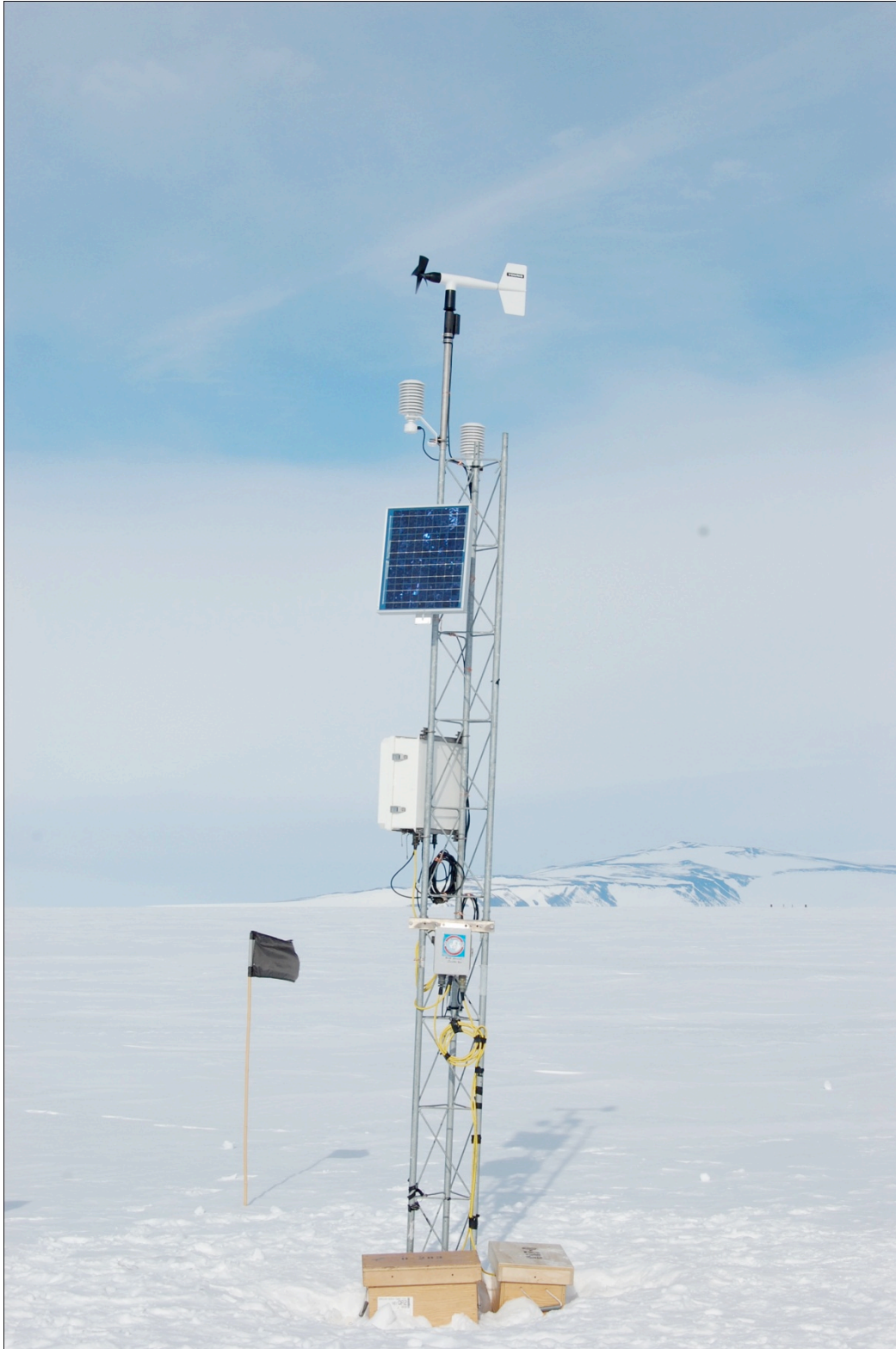
Willy Field CR1000 based AWS for testing Freewave transmitter
