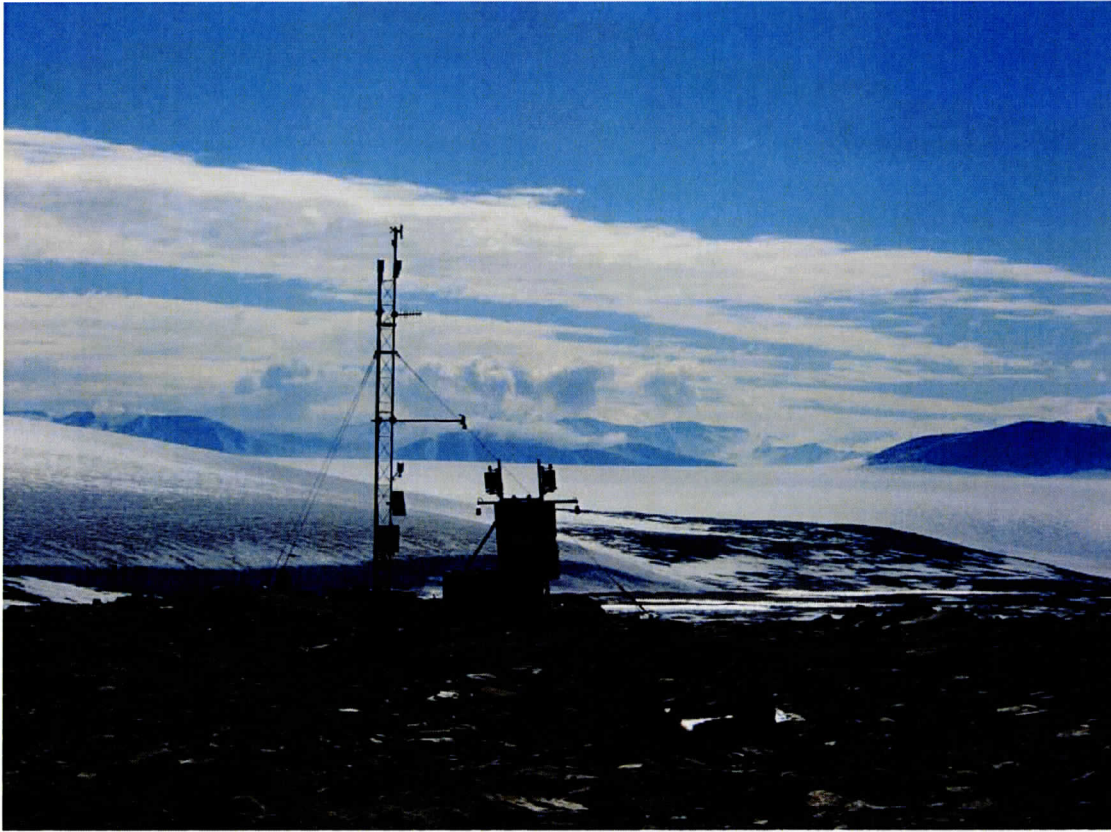
Figure 1. A photograph of the Marble Point Automatic Weather Station (AWS) ozone sensor joint system along with the UNAVCO power system. (Photo Courtesy of Lars Kalnajs)
