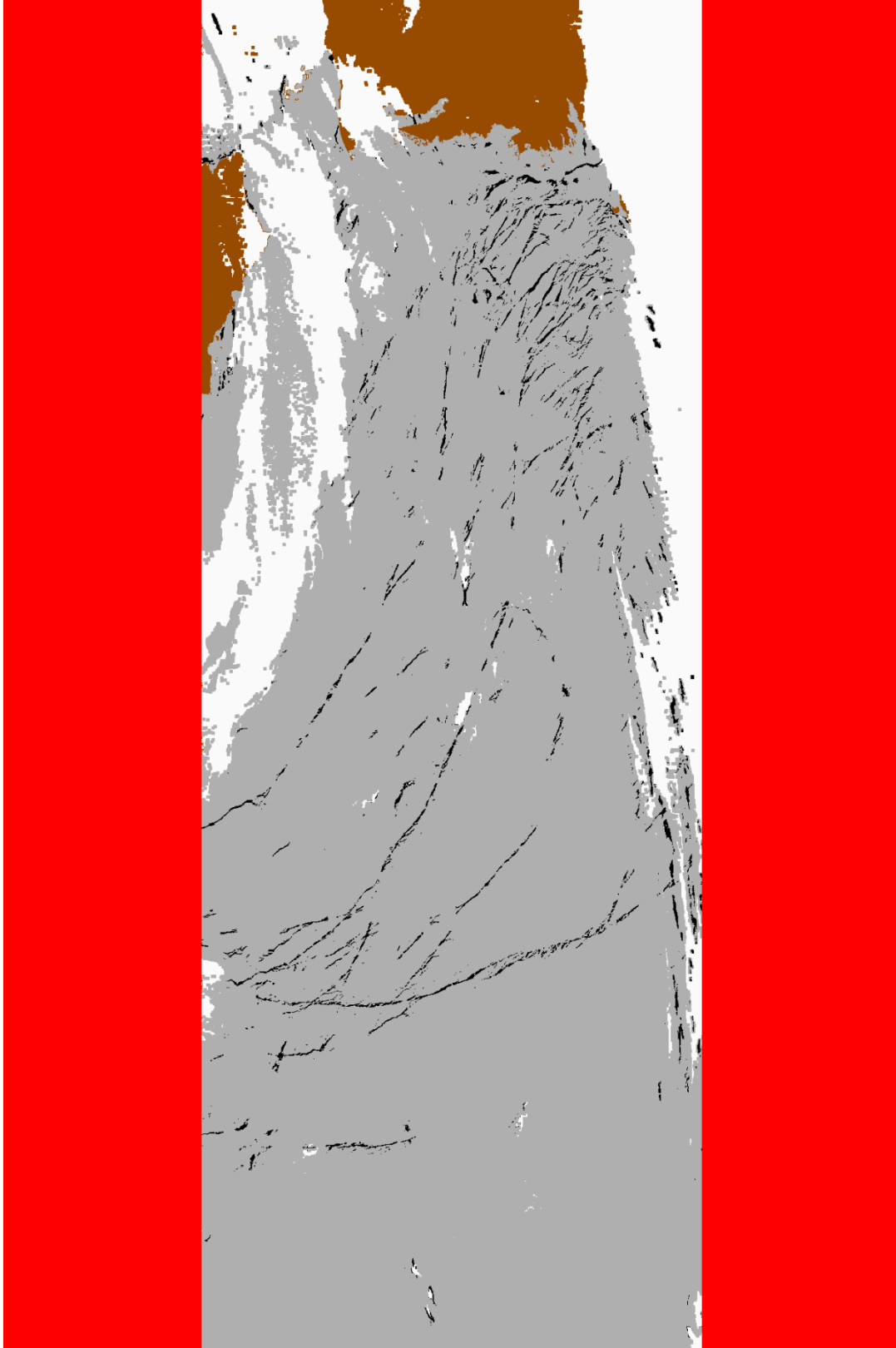
Figure 6. MODIS-TERRA potential lead mask from the case study overpass from 0545 UTC on 15 February, 2018. Potential leads are in black, clouds are white, land is brown and the scan angle block out is illustrated in red.
