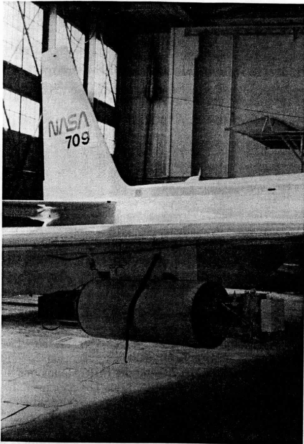
FIG. 1. The HIS instrument mounted in a wing pod used for early U-2 flights. The nose and rear sections of the pod, not shown here, are attached prior to flight. For FIRE the pod is mounted along the centerline of the fuselage of the ER-2, directly beneath the aircraft engine.
