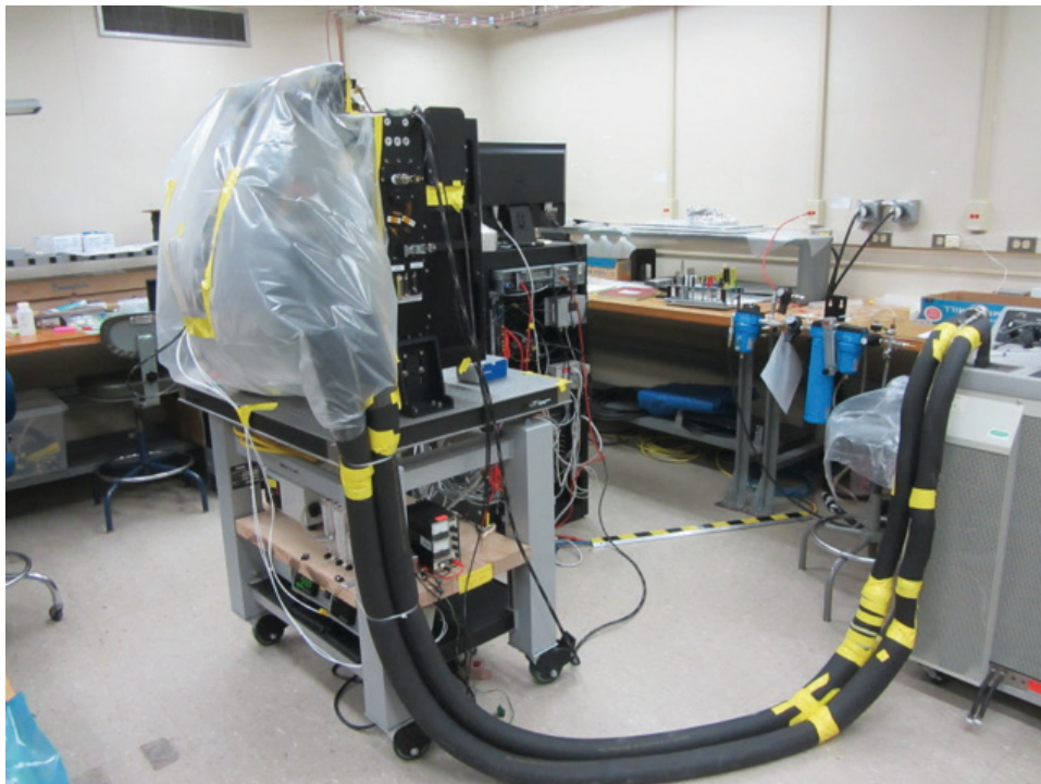
Figure 61: Stray light diagnostic tests. A recirculating chiller is used to cool the OARS and CBB to 243 K. The instrument, including the calibration and verification sources, is purged with dry air and a dew point of less than 233 K was maintained.
