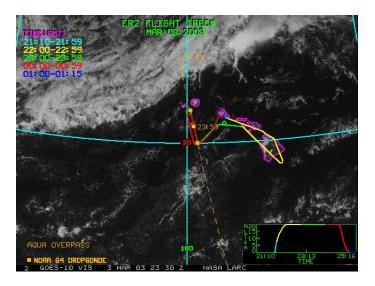
Figure 1: 03 March 2003: ER-2 Flight Track. The yellow squares indicate the locations where dropsondes were released by the G-4.
