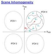
IFOV 4 contains 6 different homogeneous scenes, with an indication of their centres of gravity. The interferometer axis is in the centre of the  $X_{\text{IASI}}$ - $\gamma_{\text{IASI}}$ -plane.
