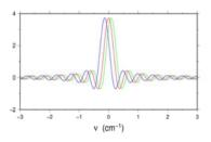
Three response functions are shown for the centre of an IFOV (red), the IFOV border closest to the interferometer axis (blue), and the IFOV border farthest from The interferometer axis (green).
