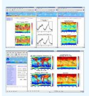
Radiance Products can be displayed for selected instruments (AIRS, AIRS co-located MODIS, IASI, AMSU...), date, and channels. The performance of the instruments are also monitored using the Principal Component Analysis (PCA) technique.
