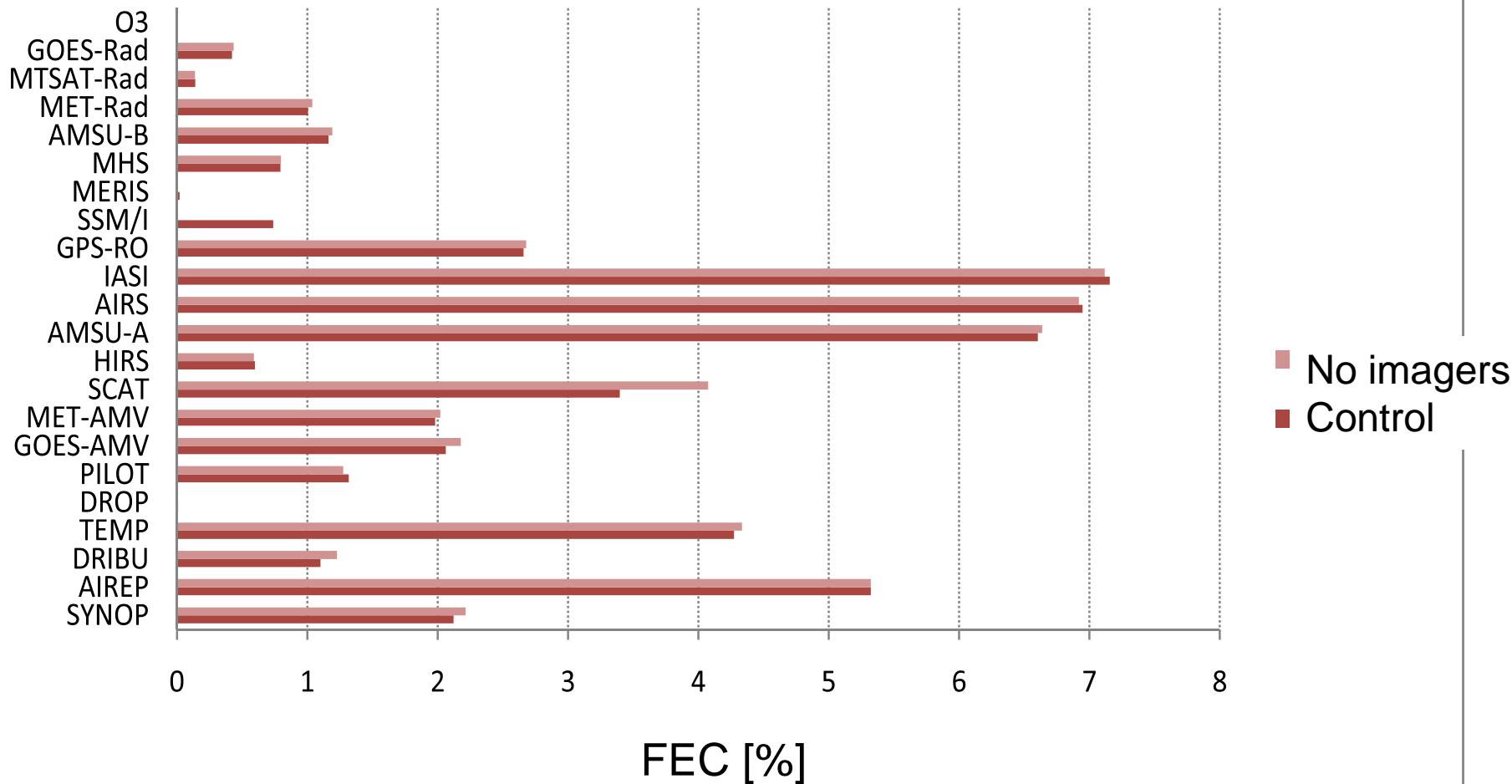
Impact of removing all-sky microwave imager assimilation (SSM/I, AMSR-E). Note little impact on sounders and conventional observations but big impact on scatterometers.
