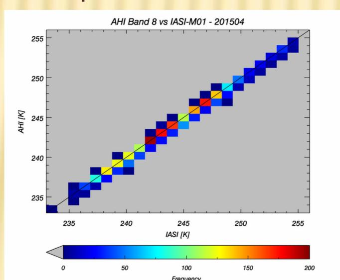
The agreement between IASI and AHI is excellent for instance in band 8, as plotted here for April 2015, with almost no dependency with the scene temperature, whether all homogeneous collocations are included (left plot) or with only IASI FoVs that are flagged as clear (right plot).
