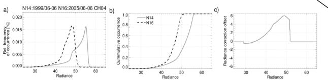
**Figure** Globally aggregated histograms of HIRS ch4 for NOAA-14 and NOAA-16 (a), also shown as cumulative histograms (b). Panel (c) shows the radiance dependent correction offset which is to be applied to NOAA-14 channel 4 to mimic NOAA16.
