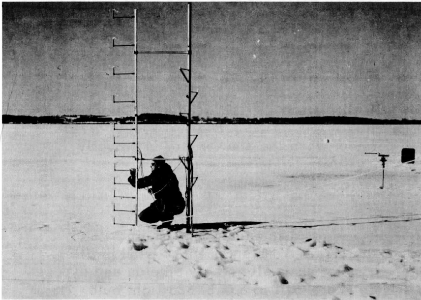
Fig. 10. Winter installation of anemometers.
