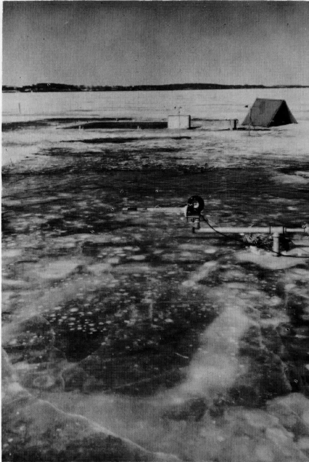
Fig. 5. Experimental site, 24 February 1963, facing north. 0.3 cm temperature sensor visible in ice in immediate foreground. Net radiometer on its stand in center of picture.
