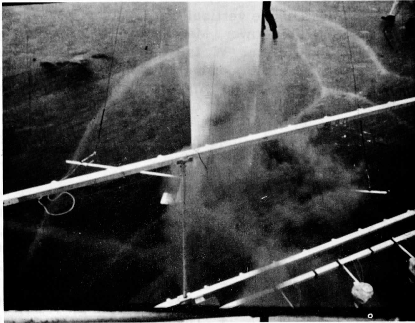
Fig. 8. Smoke plume passing a circular cylinder of 56 cm diameter. The smoke is being emitted from a smoke grenade on the ice surface. The wind speed at height of 2m is about 1 \text{ m sec}^{-1} .
