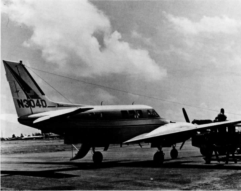
Figure 4. The Queen Air aircraft of NCAR. This aircraft was instrumented with Eppley pyranometers on top and bottom of the aircraft. The upper instrument was mounted on top of the fuselage between the two small air scoopers. The lower instrument was mounted on the rear (flat) deck just forward of the tail assembly.
