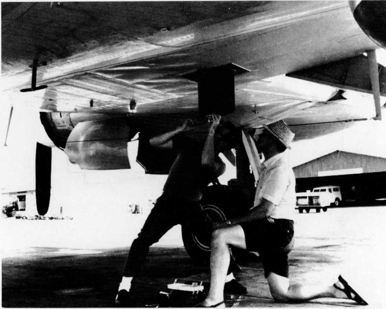
Figure 7. An Eppley precision pyranometer is being installed on the bottom of an RFF DC-6 aircraft.
