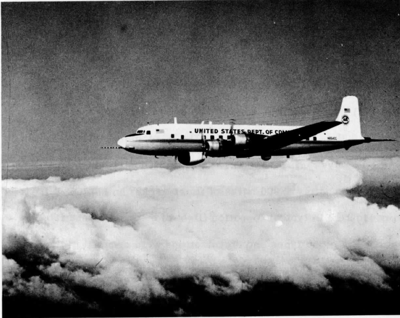
Figure 2. A DC-6 of the Research Flight Facility of ESSA is shown on a flight mission for the University of Wisconsin Radiation Measurement Program. Precision radiation sensors were installed on top and bottom of this and other RFF aircraft. The normal mode of observation was to fly one aircraft directly over the other separated by many thousand feet, in order to measure the absorption of sunlight and the layer of atmosphere between the two aircraft. Measurements from 1 to 12,000 feet were obtained in this manner.
