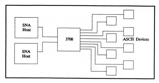
As many as nine ports can be defined for ASCII hosts. Each of these ports can connect to separate hosts, or multiple ports can connect to the same host, depending on the host.
