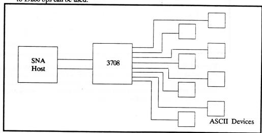
As many as two ports can be defined for SNA hosts. Each of these ports can connect to separate hosts, or can connect to the same host.
