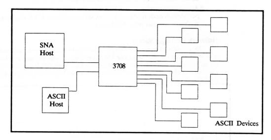
When a 3708 port is connected to an SNA host, multiple end-user devices can communicate at the same time over that one line. When a 3708 port is connected to an ASCII host, only one end-user device at a time can communicate over that line. However, multiple devices can communicate at the same time with an ASCII host if each device has a separate line to the host.
