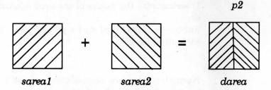
The left sides of sarea1 and sarea2 comprise the final image. You may need to do several AA commands to obtain the desired result. For two horizontally split images, p1 defines the line number where the split occurs; p2 must be larger than either area's line number.
