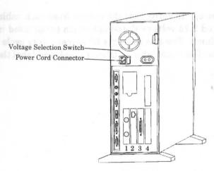
The voltage-selection switch is located immediately to the right of the AC power cord connector, as shown in the drawing at the left. If your voltage is between 90 VAC and 137 VAC check to see that 115 is visible on the switch; if your voltage is between 180 VAC and 265 VAC, check to see that 230 is visible on the switch.
