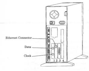
Connect the Data and Clock inputs shown in the drawing at the left. This completes the SDI installation process.
