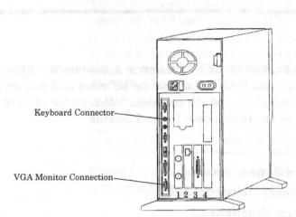
You can use any color or monochrome VGA monitor by connecting its data cable connector to the 15-pin D-connector located at the bottom-left corner of the computer, as shown in the drawing at the left.
