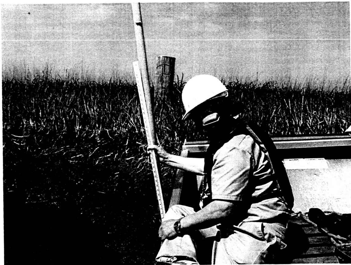
Fig DCS-3. Oscar making measurements at DCS#4. Note eroded mud bank of background and position of fence row post to ongoing erosion. (Photo DCS_3_pipe.jpg)
