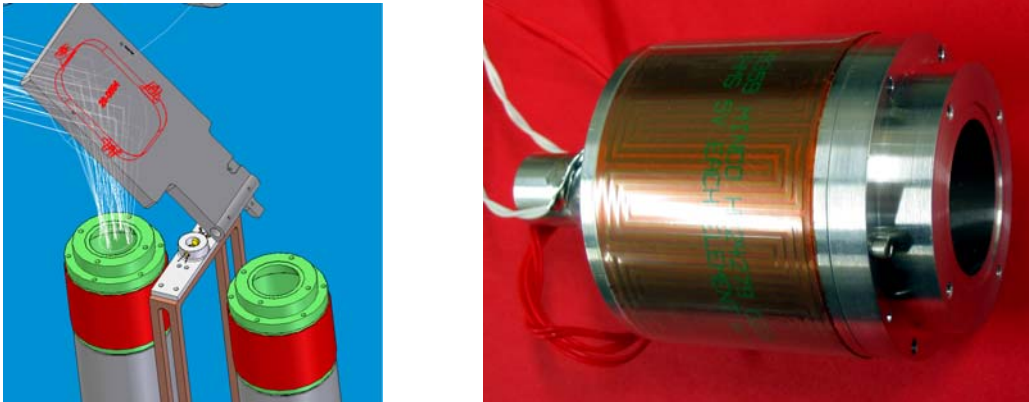
Figure 6. The left-hand panel illustrates two blackbodies and a visible flood source mounted on the same linear slide. One source at a time is correctly positioned under the flip-in mirror. The right-hand illustration is a photo of the UW-SSEC engineering model of the GIFTS blackbody. The blackbody aperture is 1.00 inches in diameter, the width of the cylindrical body is 1.76 inches in diameter, and the total cavity depth is 3.06 inches.
