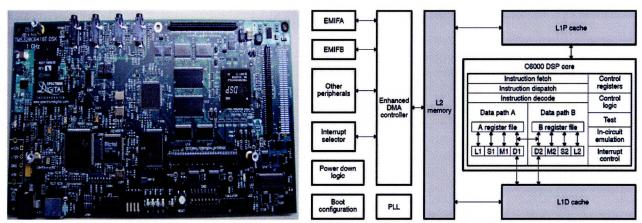
Texas Instruments' TMS320C6416 DSP board. TMS320C6416 two-level cache-based architecture. Figure 1. A memory-limited DSP version of 3DWT-RVLC code is implemented on Texas Instrument's TMS320C6416 DSP board to explore its feasibility for real-time satellite rebroadcast processing.
