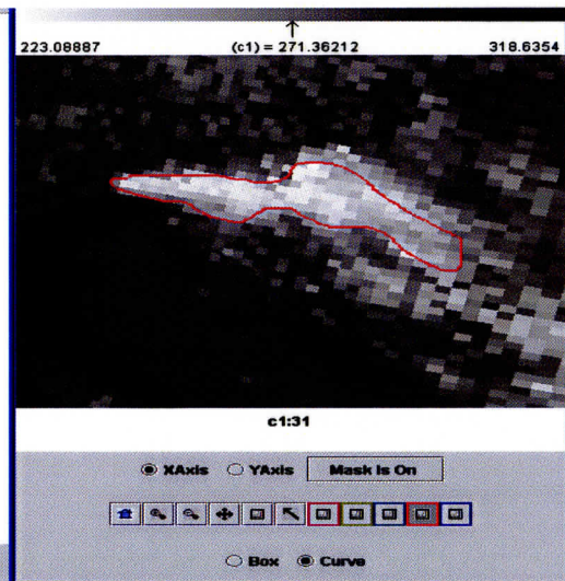
Figure 15.14: Scatter plot (left) of [BT31 (11 \mu\text{m} )] on the x-axis and [BT31 (11 \mu\text{m} ) - BT29 (8.5 \mu\text{m} )] on the y-axis. Cloud in BT31 image (right) shows negative [BT31-BT29] values in scatter plot, suggesting ice cloud.
