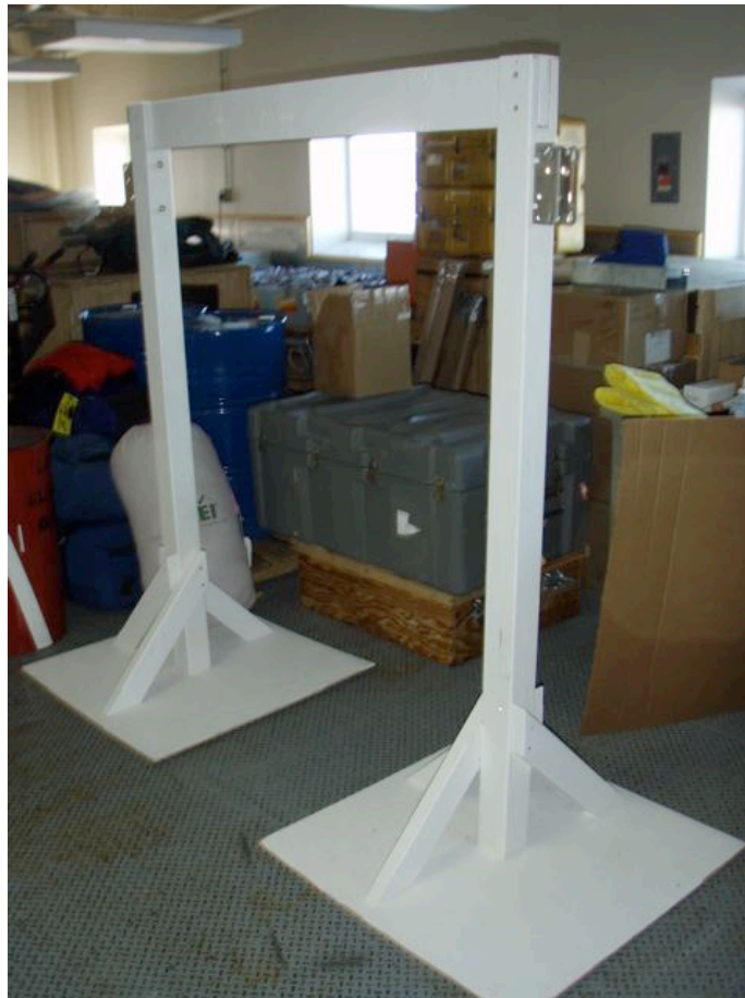
Figure 2. Mounting platform for radiation shield/temperature sensor testing.
