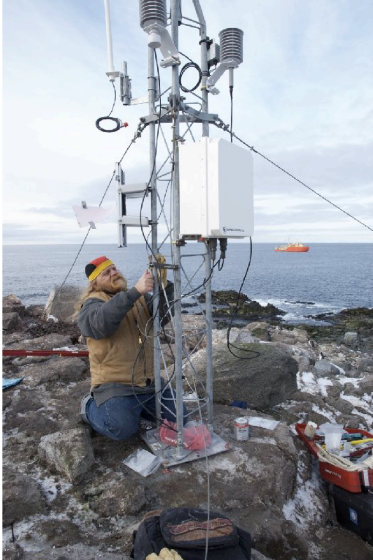
Image A33: W. Kevin Pedigo (Sr. Marine Computer and Instrument Specialist) on the ARSV Laurence M. Gould installing AWS at Hugo Island
