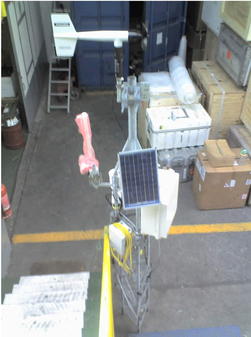
Image A32: AWS for Hugo Island under test in Punta Arenas
