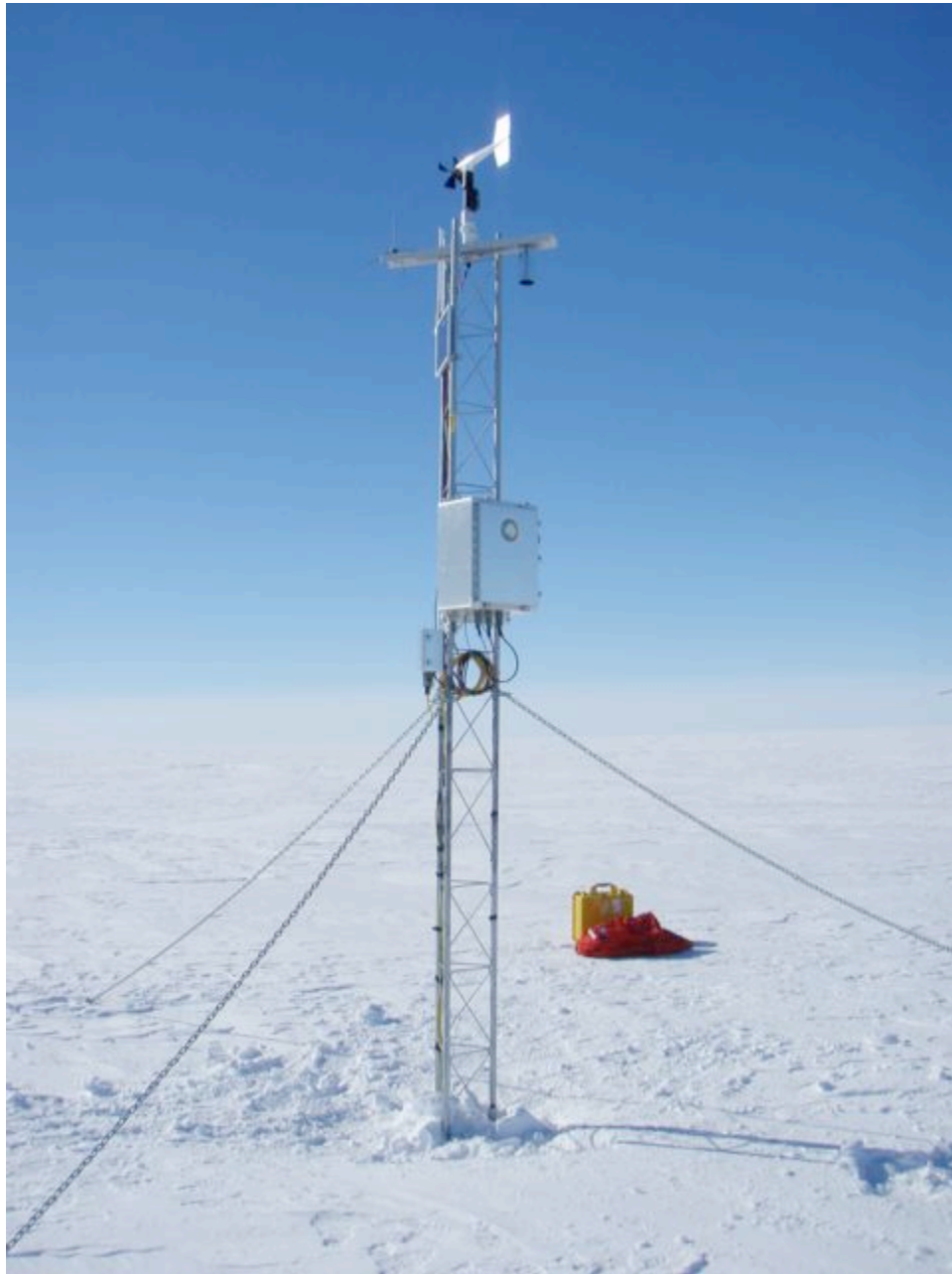
Image A8: Lorne AWS on November 4, 2008 after servicing
