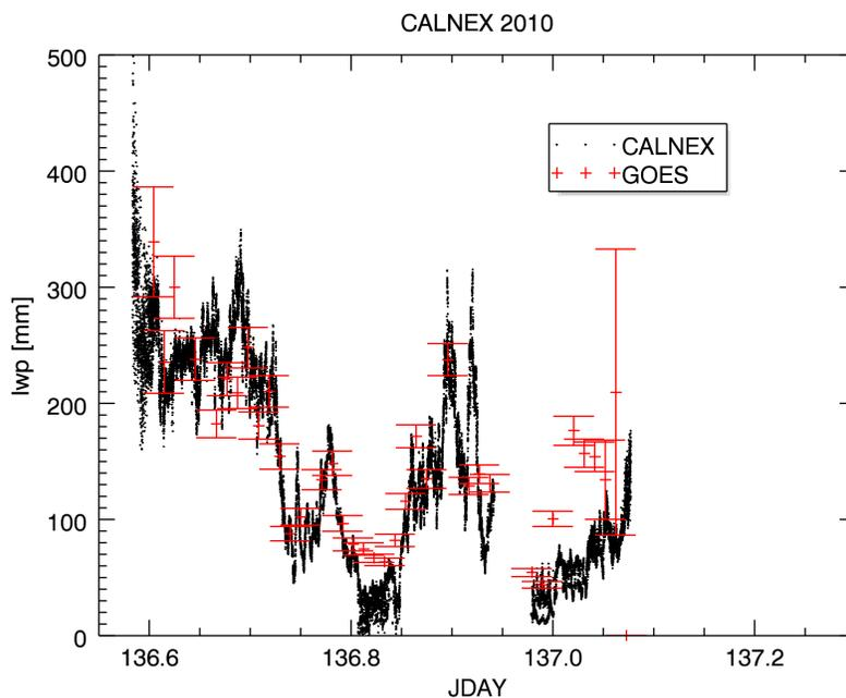
**Figure 3 Validation of Liquid Water Path with ground-based Solar Spectral Flux Radiometer instrument (SSFR) during CALNEX 2010 project**
