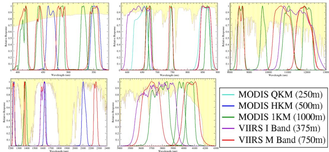
**Figure 44** Government team “best” sensor level in-band Relative Spectral Response (RSR) for VIIRS Flight 1 instrument, shown with Aqua MODIS RSR. The VIIRS government team independently derived VIIRS RSR to verify industry RSR specification compliance, as well as to improve the RSR information content. Color coded legend applies to all panels. Model based atmospheric extinction is represented by the yellow background of each panel.
