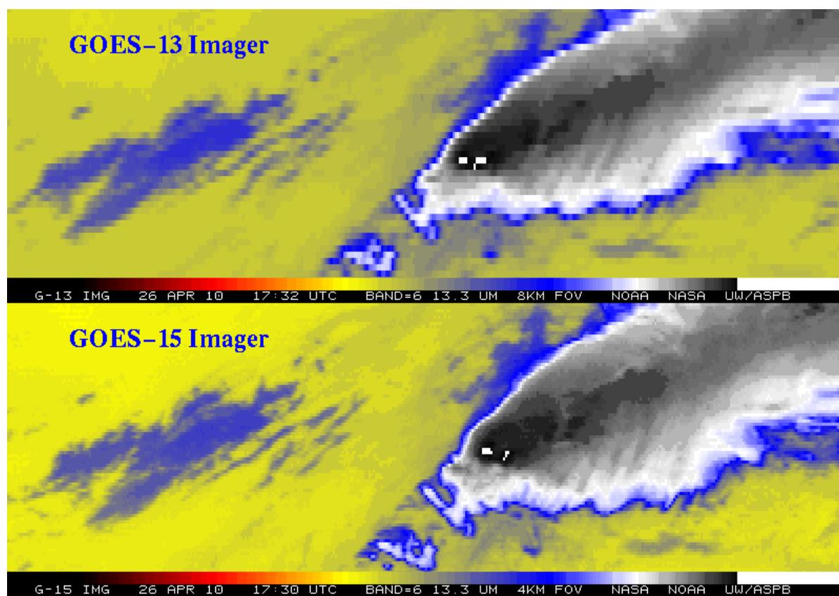
Figure 1 A comparison of GOES-13 (8 km Instantaneous Geometric Field of View) and GOES-15 (4 km) Imager Band 6 (13.3µm) on 26 April 2010. Note the 'cleaner' image from GOES-15.
