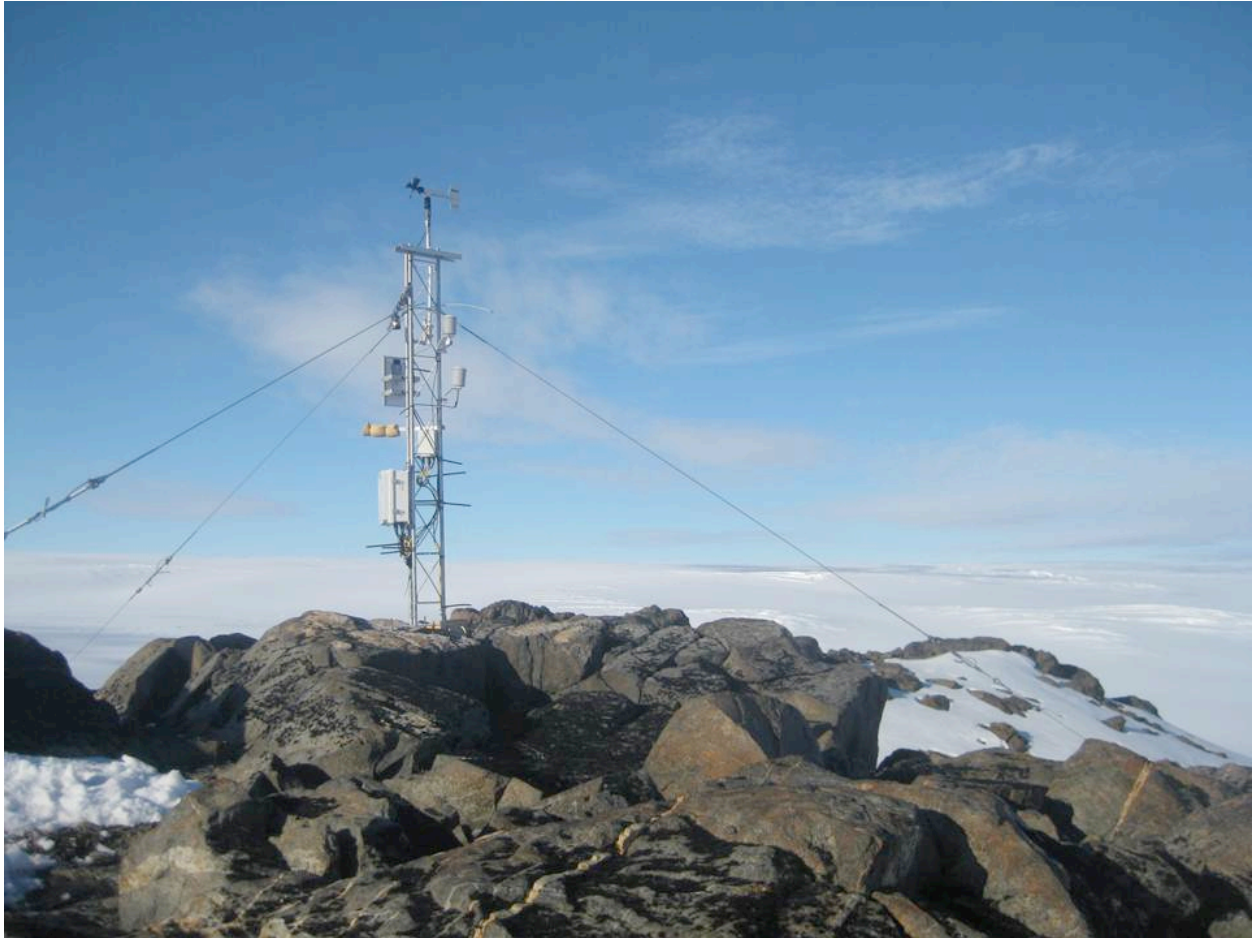
Installation of CR1000 AWS on Thurston Island on January 19 th , 2011 by David Holland's field team
