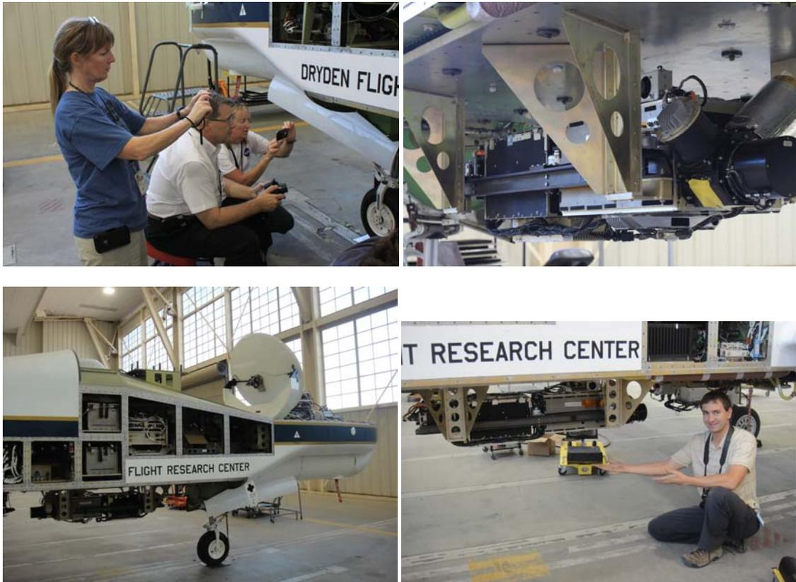
Figure 7. Final S-HIS installation on the NASA Global Hawk 872 (August 2011 at DFRC).
