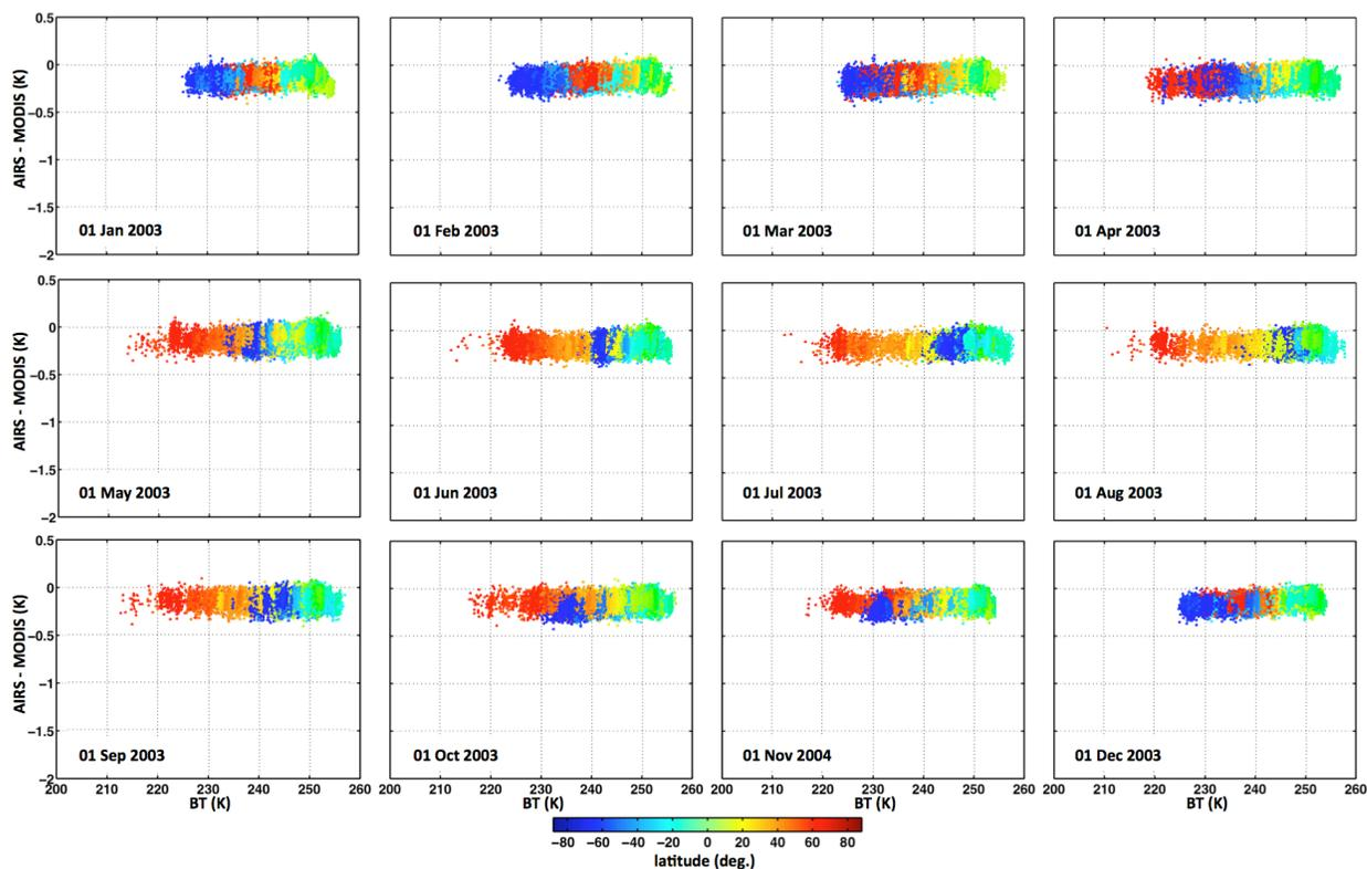
Figure 2: Same as the previous figure, but the AIRS–MODIS data are convolved after shifting the nominal MODIS SRF by  $0.8 \text{ cm}^{-1}$ .
