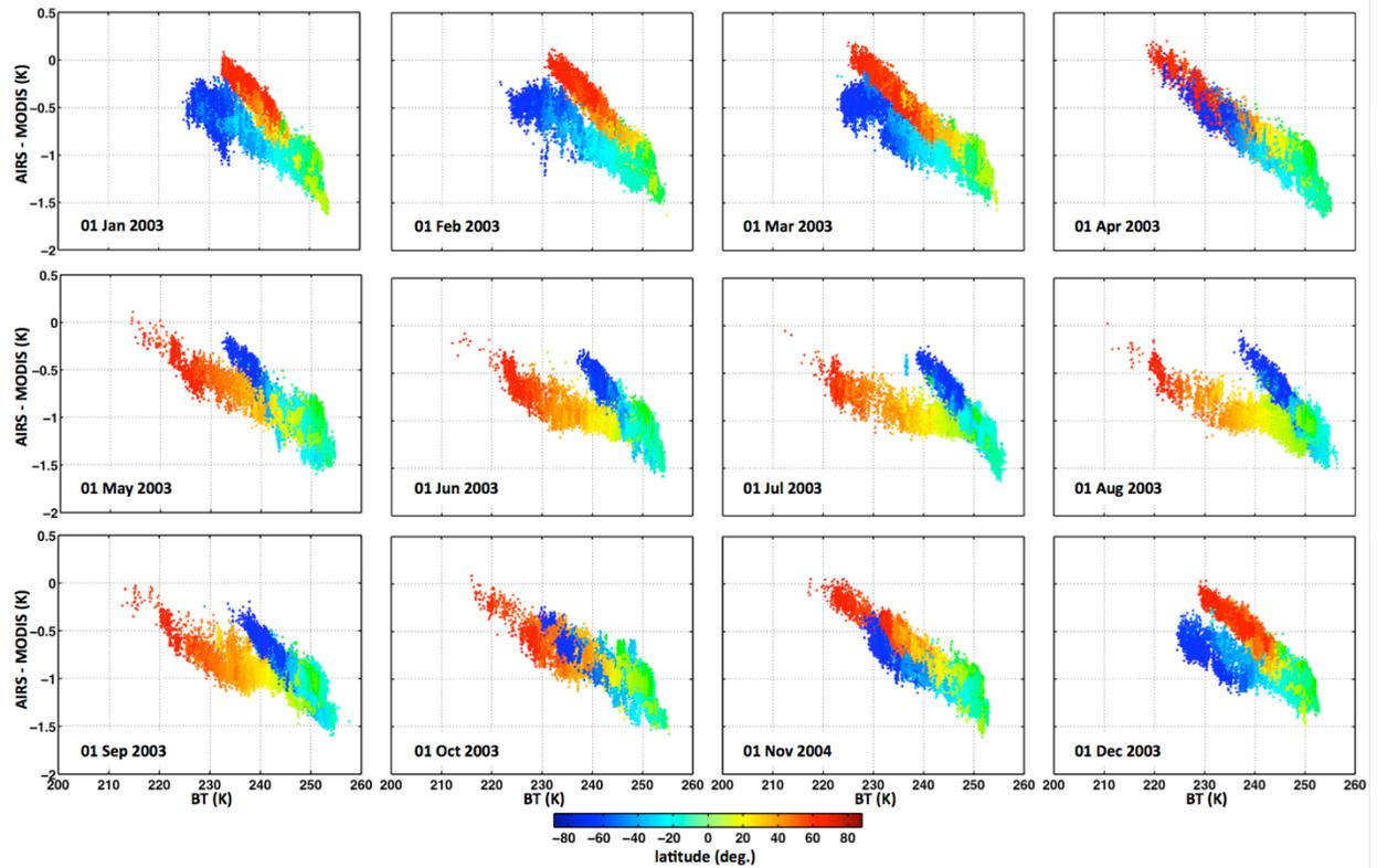
**Figure 1:** The (AIRS–MODIS) brightness temperature differences (BTD) are shown as a function of 11- $\mu\text{m}$  scene brightness temperature (BT). The (AIRS-MODIS) BTD are calculated with AIRS data convolved using the nominal MODIS SRF (i.e., unshifted). The BTDs are color coded as a function of latitude, with red points coming from the high latitudes in the northern hemisphere and the blue points come from high latitudes in the southern hemisphere.
