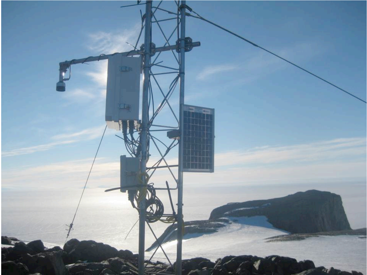
Installation of CR1000 AWS at Bear Peninsula on January 14 th , 2011 by David Holland's field team
