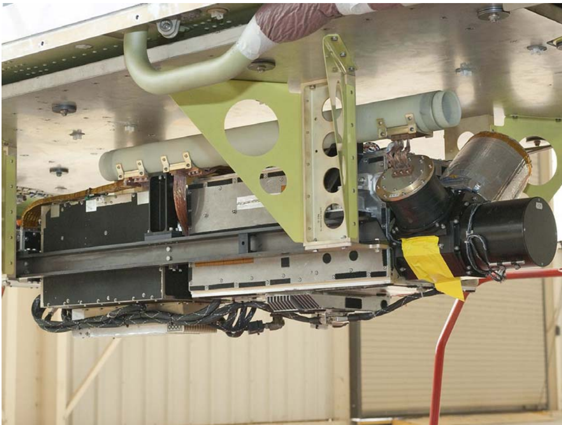
Figure 8: The Scanning HIS integrated to the Global Hawk with the heat straps (4 of 5 are visible) in place and connected to the rigid segment of the outside air flow tube.
