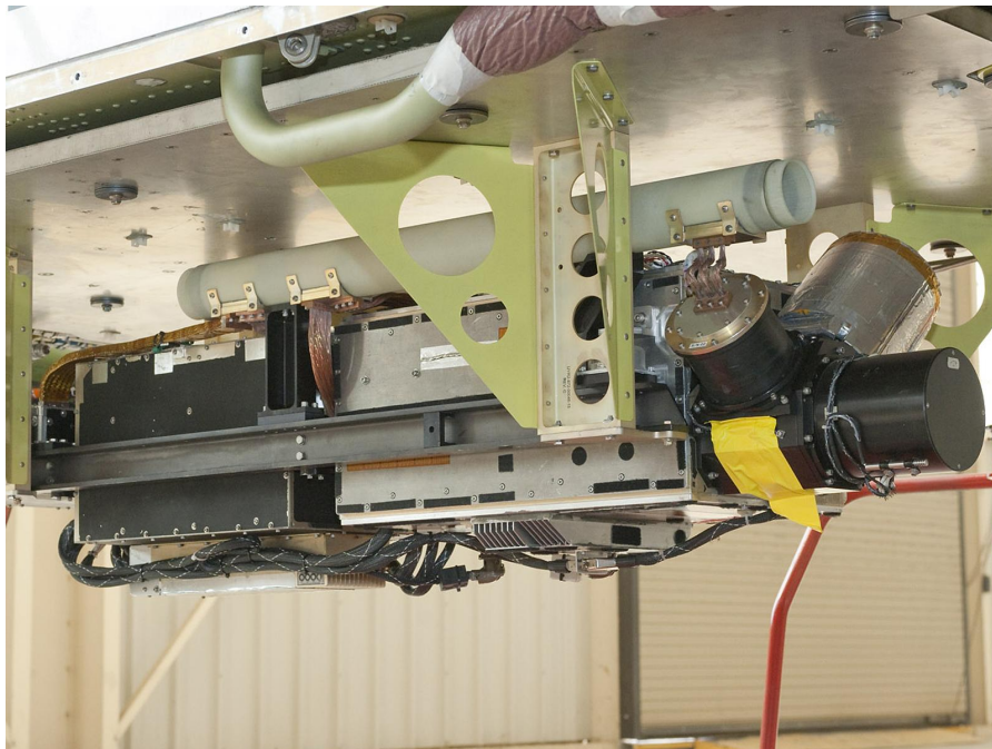
Figure 5: The Scanning HIS integrated to the Global Hawk with the heat straps (4 of 5 are visible) in place and connected to the rigid segment of the outside airflow tube.
