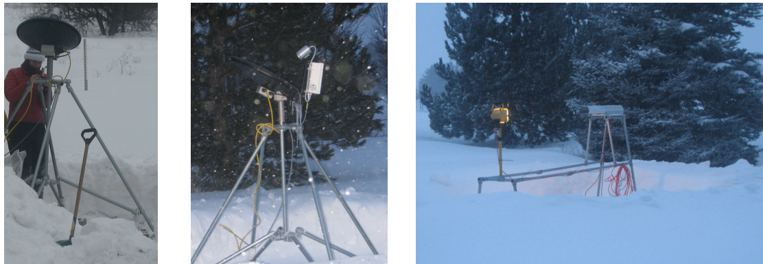
FIG 1: Micro Rain Radar (left and center) and Precipitation Imaging Package (right) deployment at the Marquette, MI National Weather Service Forecast Office during January 2014.
