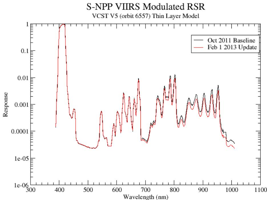
**Figure CCM1. SNPP VIIRS band M1 showing baseline and modulated (Feb 1, 2013) Relative Spectral Response. VIIRS Reflected Solar Band RSR are modulated by darkening of the VIIRS RTA mirrors due to tungsten contamination. This causes a noticeable relative reduction in M1 response beyond 600nm.**
