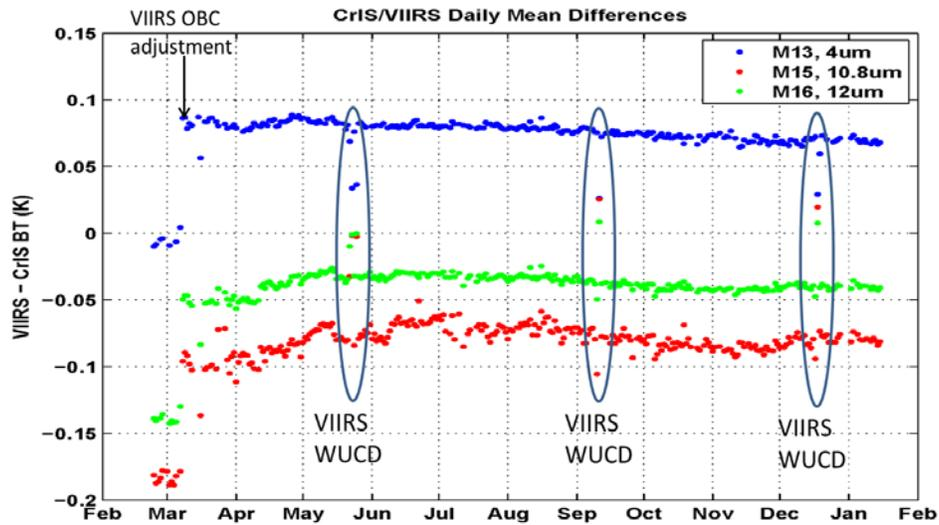
Figure B-2. VIIRS-CrIS spectral radiance differences from March 2012 – Jan 2013 demonstrating excellent stability in VIIRS (and CrIS) radiometric calibration. VIIRS calibration was adjusted in March 2012, improving the comparison to CrIS. VIIRS Warmup-Cooldown (WUCD) events are planned blackbody (OBC) exercises and do not represent an anomaly but do demonstrate a dependence of VIIRS calibration on the operating temperature of the OBC (see item 3 in text).
