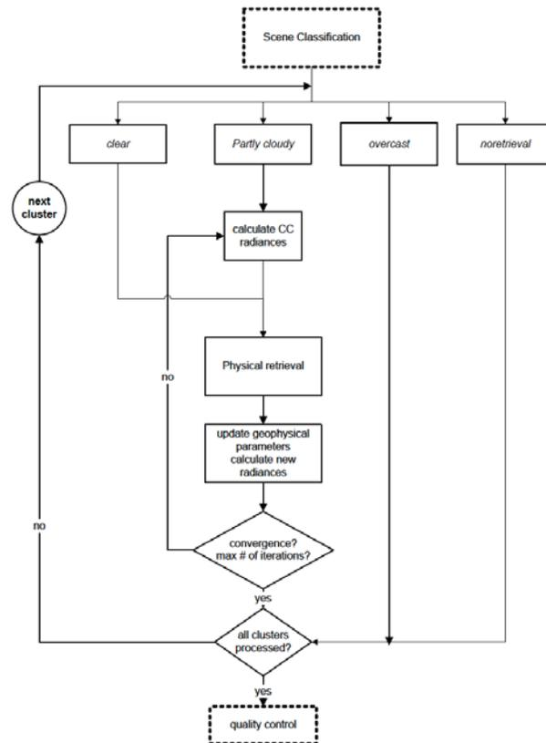
**Figure 11. Joint microwave and infrared retrieval flow chart.**
