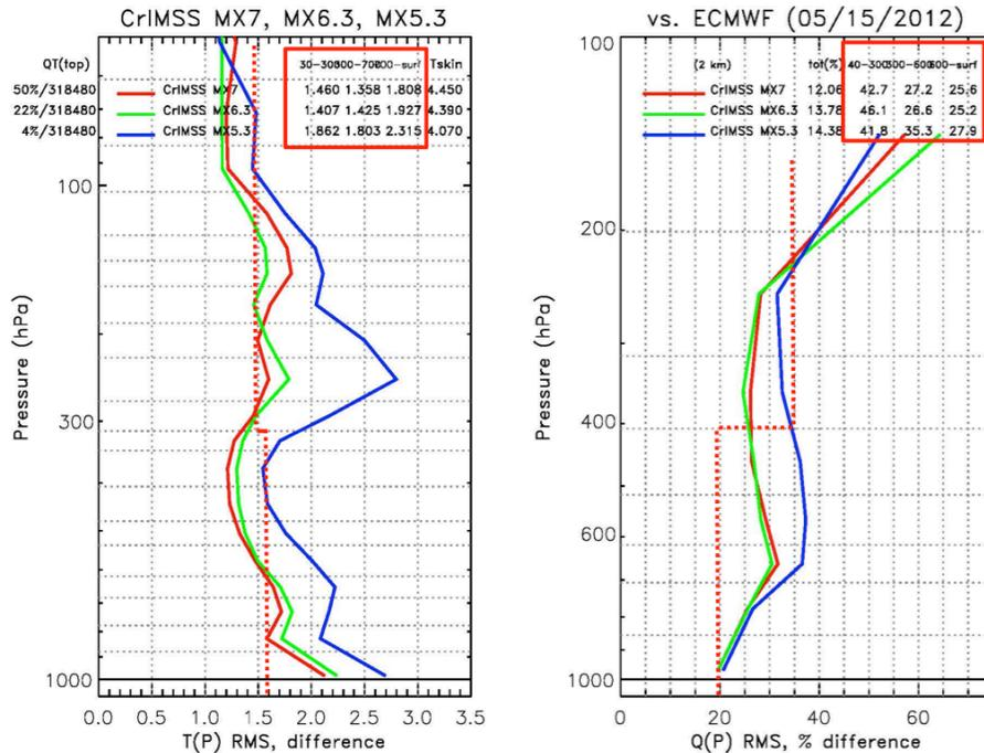
Figure 12. Provisional maturity evaluation of Mx5.3 (past), Mx6.4 (current), and Mx7.1 (future) performance of CrIMSS algorithm versions implemented for IDPS compared to JPSS requirements (from Chris Barnet, NOAA).
