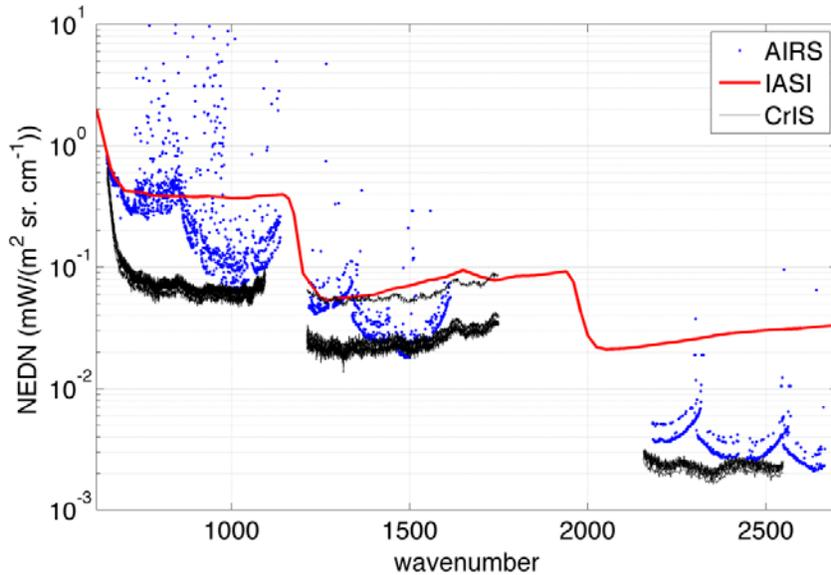
Figure 2. Comparison of CrIS radiance noise (NEDN) to that for AIRS and IASI. Note that in the important 15 micron band region, CrIS noise is about 4 time smaller than both AIRS and IASI. Also noteworthy is the excellent performance even in the shortwave band (2150 to 2600  $\text{cm}^{-1}$ ). This comparison is made for warm scenes, but even for cold scenes the shortwave noise performance is comparable to that of AIRS.
