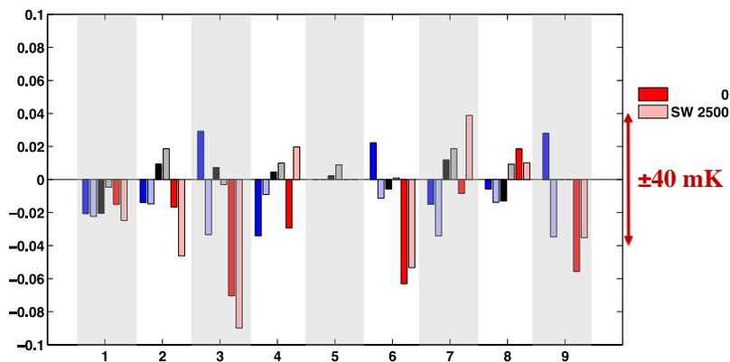
Figure 4. On-orbit brightness temperature comparisons among CrIS nine individual FOVs composing each 50x50 km FOR for six sample wavenumbers. Note that most differences are less than  $\pm 20$  mK. The exception are SW pixels 3, 6, and 9, an anomaly that is still being studied. In general, these relative comparisons that inherently include some errors from the on-orbit comparison process are excellent and consistent with the expectations of Figure 3.
