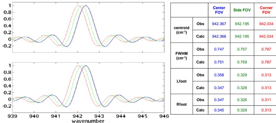
Figure 8. CrIS Instrument Line Shapes measured with a CO<sub>2</sub> laser compared to calculations.
