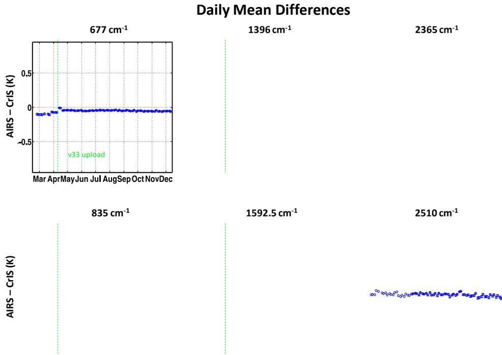
Figure 6. Temporal stability of AIRS minus CrIS differences for six sample wavenumbers. The small jog in April was caused by an upload of new calibration parameters for CrIS. Note that the differences are usually significantly less than  $\pm 0.2$  K.
