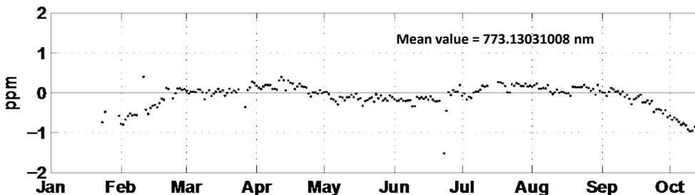
**Figure 10. Stability of the FTS sampling laser relative to the on-board Neon calibration source is on the order of 1 ppm.**
