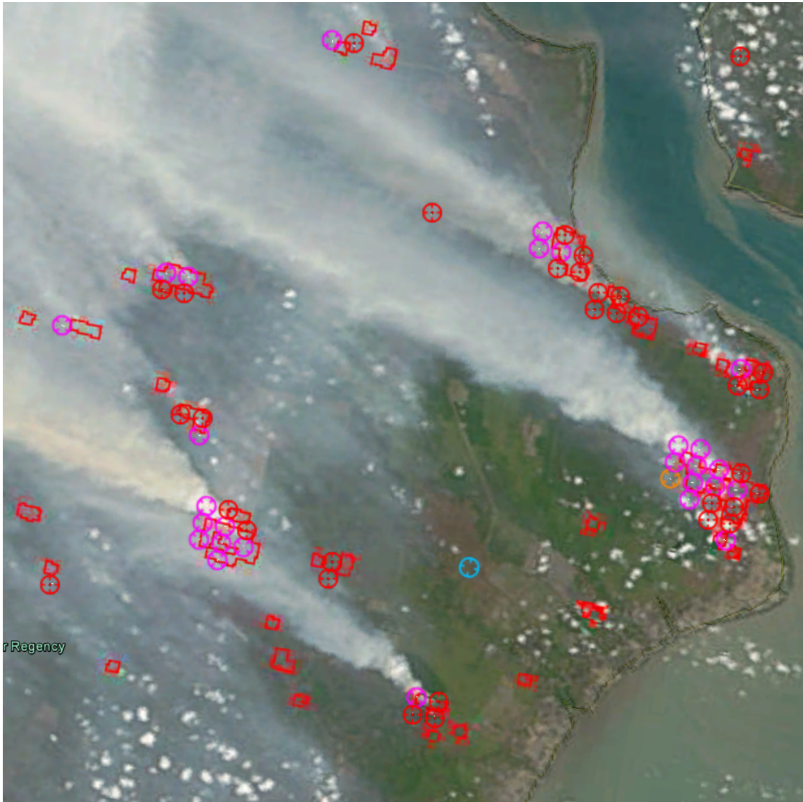
Figure 10. FDCA fire detections from Himawari-8 AHI data over Sumatra at 3:20 UTC on 24 September 2015 overlaid on MODIS Aqua imagery and fire data from 3:15 UTC. MODIS fires are red polygons, FDCA fires are red, magenta, and cyan colored targets. The two instruments agree well. This data was created before the bug affecting detections was fixed.
