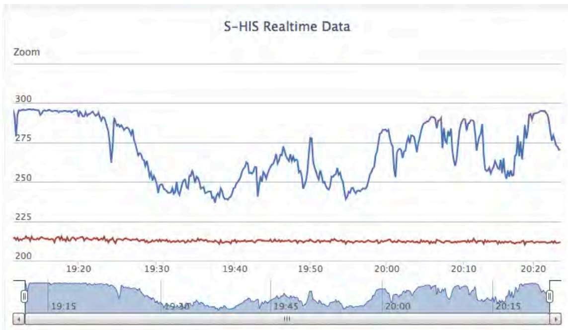
Figure 14: A new data display showing time series of realtime S-HIS brightness temperatures was tested. 895-905 \text{cm}^{-1} (blue) and 690-700 \text{cm}^{-1} (red) channels are shown above (2013-09-16).
