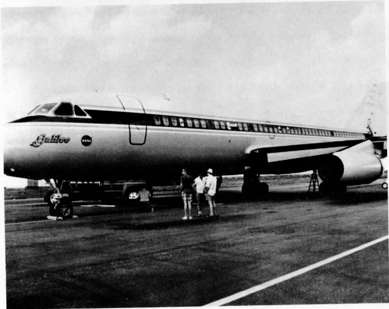
Figure 5. The NASA Convair 990 aircraft on which Eppley Laboratory has installed up and down-facing precision pyranometers. The radiation program, under Messrs. Drummond and Hickey, conducted a small number of joint flights with the (Wisconsin Radiation Program) RFF aircraft flights during BOMEX.
