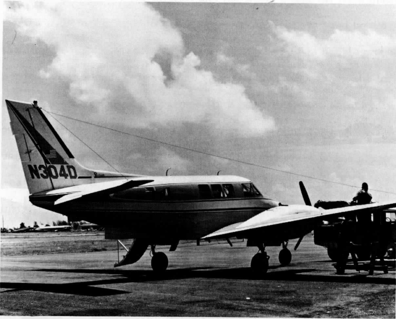
Figure 4. The Queen Air aircraft of NCAR. This aircraft was instrumented with Eppley pyranometers on top and bottom of the aircraft. The upper instrument was mounted on top of the fuselage between the two small air scoopers. The lower instrument was mounted on the rear (flat) deck just forward of the tail assembly.
