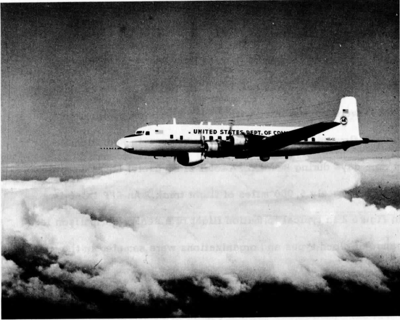
Figure 2. A DC-6 of the Research Flight Facility of ESSA is shown on a flight mission for the University of Wisconsin Radiation Measurement Program. Precision radiation sensors were installed on top and bottom of this and other RFF aircraft. The normal mode of observation was to fly one aircraft directly over the other separated by many thousand feet, in order to measure the absorption of sunlight and the layer of atmosphere between the two aircraft. Measurements from 1 to 12,000 feet were obtained in this manner.
