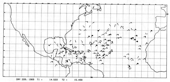
An example of cloud displacement vectors produced by WINDCO from ATS data for July 28, 1969. Cloud tracers were selected to test the WINDCO system and no effort was made to distribute vectors uniformly, nor were bad data points eliminated.
