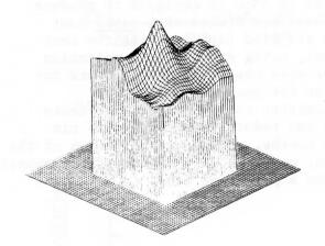
Example of a correlation matrix surface generated by the computer. The height of each grid intersection indicates the value of the correlation coefficient for a particular relative position of the two picture segments. The distance from the zero displacement position to the peak value position is the distance the cloud has moved between the two pictures.
