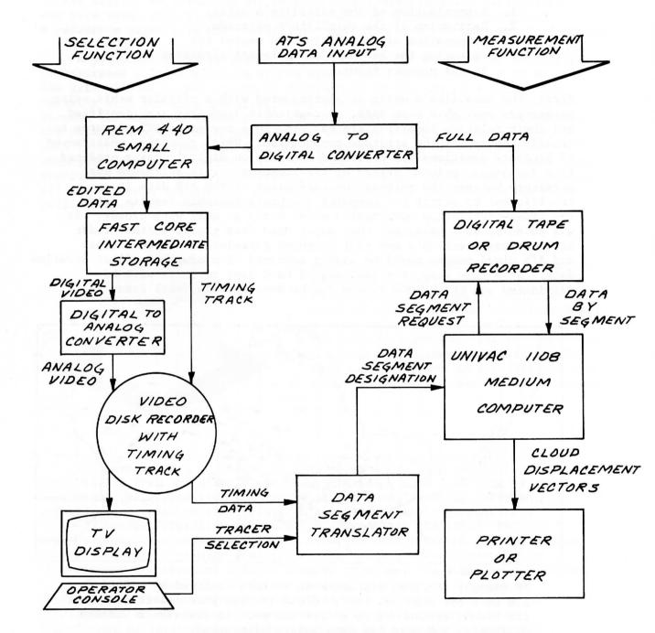
The prototype WINDCO system being developed by SSEC uses an operator to select individual tracer clouds from a TV picture and a computer to perform precision cloud displacement measurements. All video equipment is assembled from standard commercial TV components. The system is designed to produce 20 highly accurate cloud displacement vectors per minute at a cost of about 10 cents per wind.
