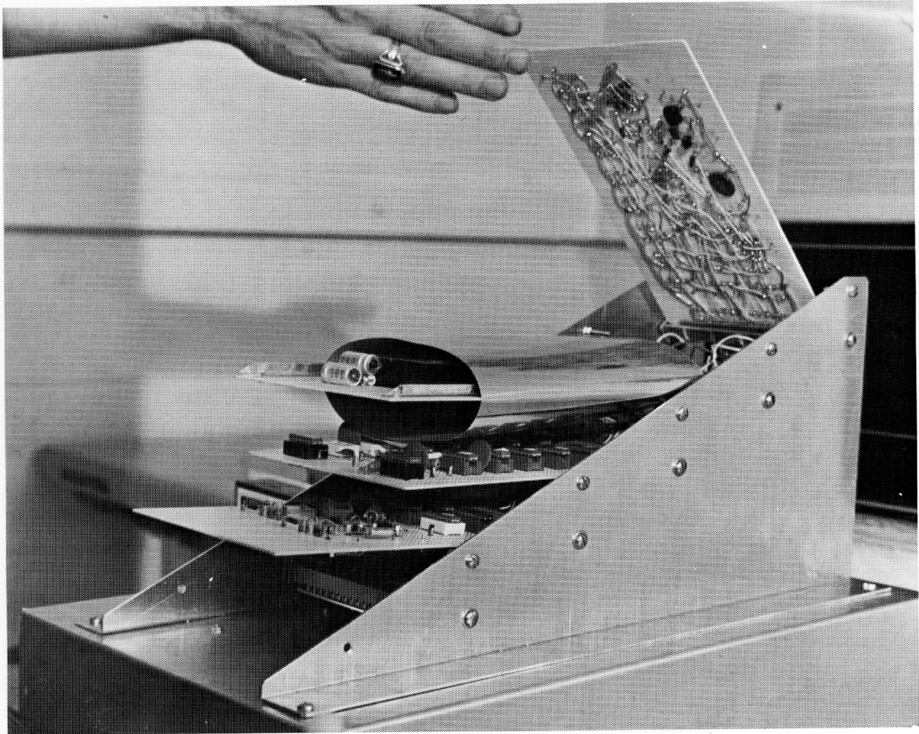
Figure 17. Breadboard Electronics. The heart of the McIDAS display system is the fast core, a set of parallel shift registers which store digital image data line by line as it comes from the computer and, when the videodisk has rotated to the proper position, spits the line out at a 12 MHz word rate through a D/A converter to be written on the disk. Timing is preserved to better than 1/4 pixel through use of an optical tachometer, and gated oscillator, so that every pixel on every line of the TV image has a fixed angular position on the disk. A cursor is displayed on the TV screen to reference the exact line and element number of any point in the image.
