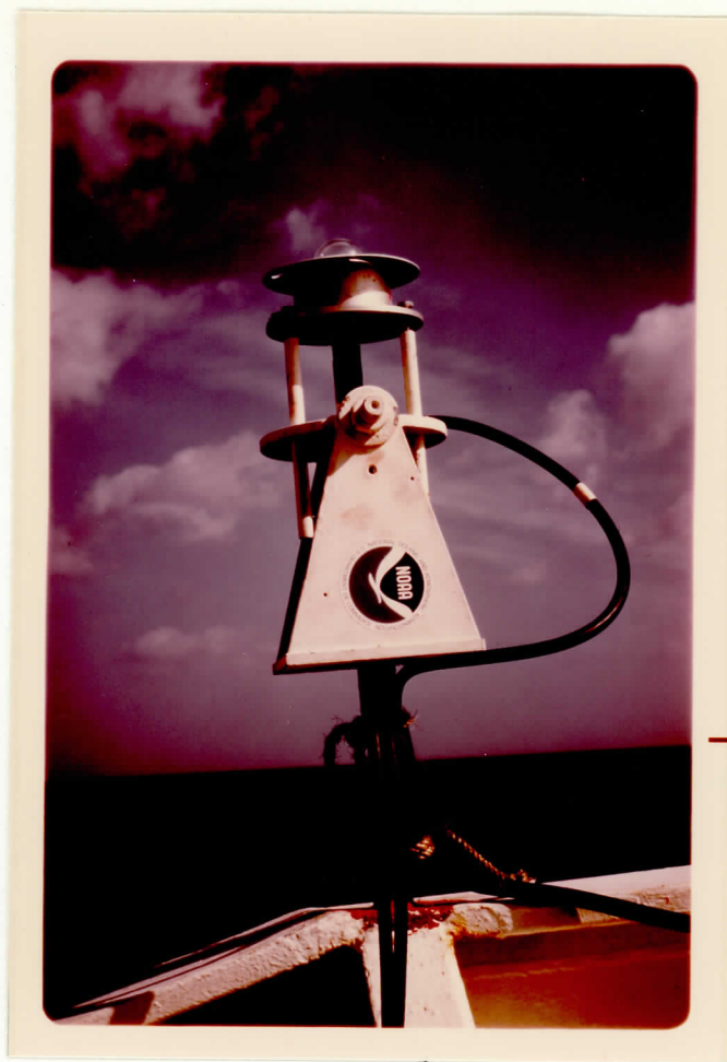
Figure 16 Deck Mounted Radiometer (Eppley PSP Uplooking Precision Pyramometer) Sea Air Interaction Laboratory
