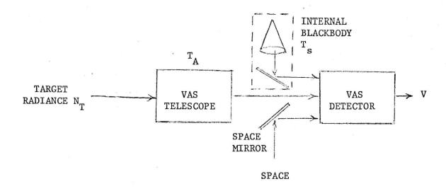
TARGET Space, earth, or equivalent external blackbody. VAS TELESCOPE Scan mirror, primary telescope, and field lens. VAS DETECTOR Relay optics (excluding field lens), detectors, and electronics. Final output is a voltage signal V. INTERNAL BLACKBODY Blackbody cone and gold mirror at ambient temperature. SPACE MIRROR Mirror introduced into optical path to provide a space view which bypasses the VAS telescope.
