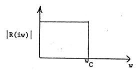
various tradeoffs come into consideration. One common criterion, called the maximally flat criterion, is that as many of the derivatives of |R(iw)| at w=0 as possible should be equal to zero. Application of this criterion leads to Butterworth filters, which have monotonically increasing attentuation, good phase characteristics and low passband losses, but the cutoff is not sharp.
