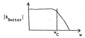
The maximally flat phase criterion requires that derivatives of the phase angle of R(iw) at w = 0 beyond the first derivative should be zero (1<sup>st</sup> derivative of  $\phi$ ,  $\frac{d\phi}{dw}$ , is called the delay).
