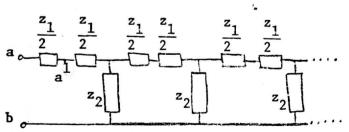
Then the impedance across  $a^1b$ ,  $z_0^{\ 1}=\frac{L}{C}-\frac{w^2L^2}{4}$ . Now there are two interesting cases: (1) if  $w^2<\frac{4}{LC}$  then  $z_0$  is real and continuous absorption of energy occurs (ie. the current penetrates far down the line) or (2) if  $w^2>\frac{4}{LC}$  then  $z_0$  is imaginary and we see no such propagation.
