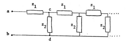
represented by  $\mathbf{z_0}$ . To determine  $\mathbf{z_0}$  we notice that this infinite network is unchanged if one more section is added to the front end, thus
