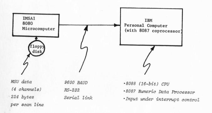
Figure 1: Microprocessor test configuration (version 2).
