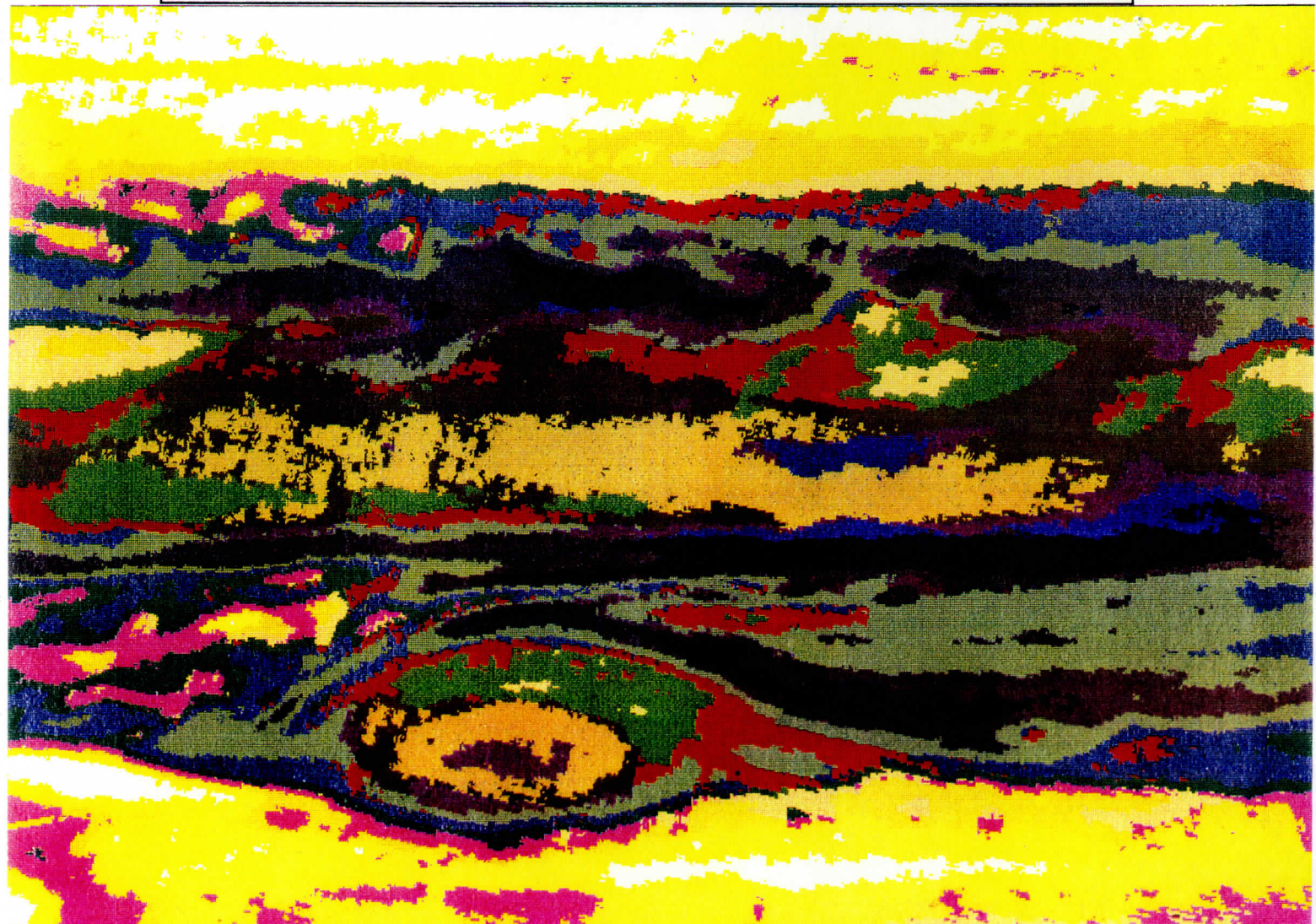
Figure 5. An example of multispectral classification using four bands. Shown are distinct spectral classes in a region of Jupiter as derived from Voyager images acquired in ultraviolet, blue, orange and green filters.
