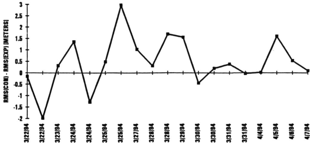
Fig. 3. Comparison of RMS errors (verified against rawinsondes) for CRAS model 72 hr forecasts of 400 mb heights for 19 cases in March/April 1994, expressed in terms of RMS(CON) minus RMS(EXP). Positive impact of the water vapor winds (EXP) is indicated in cases with points above the zero line. A few of the days contain multiple data sets (00 and 12 UTC).
