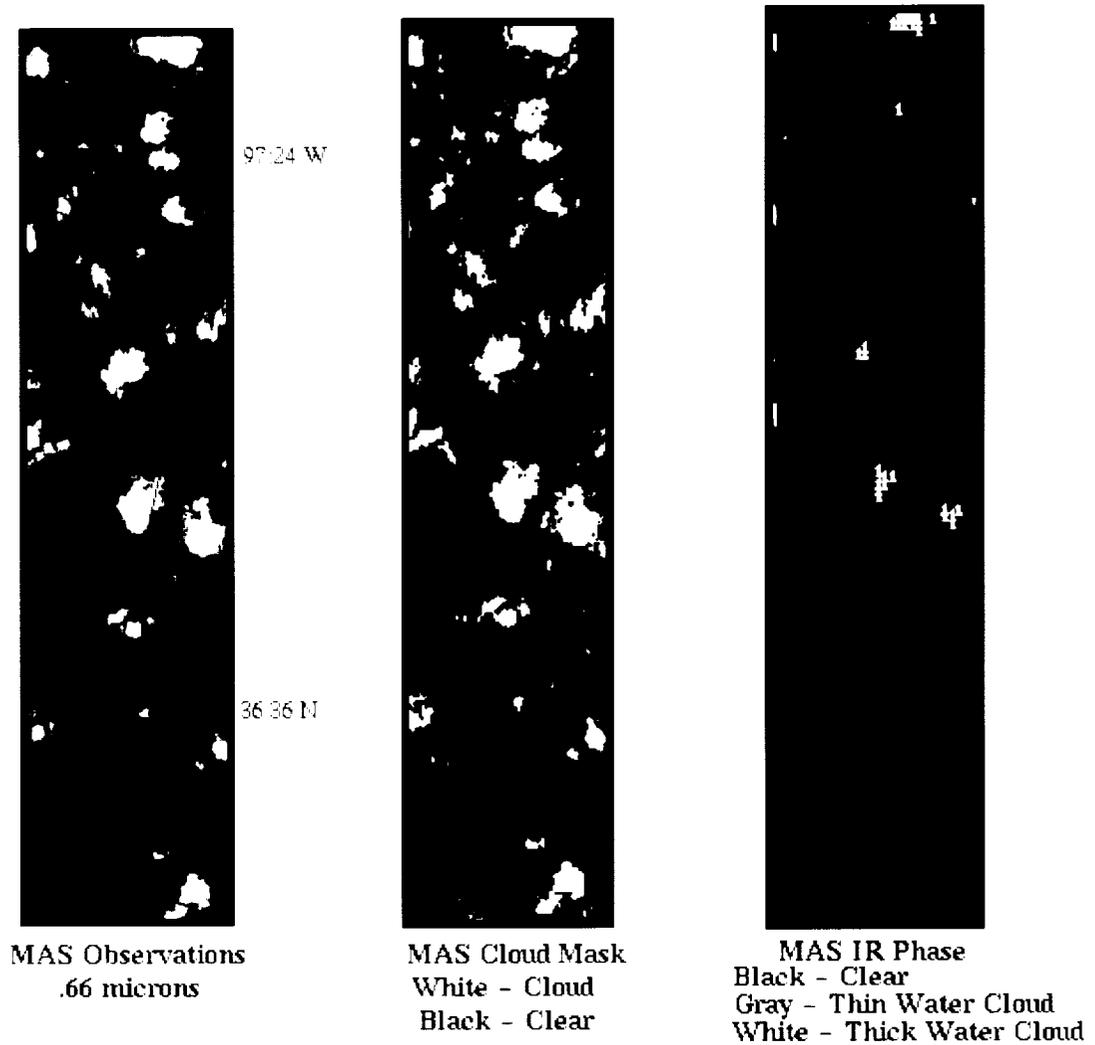
Figure 6. Example of MODIS algorithm tests using MAS data. The left scene is actual visible channel observations while the center and right panels are products. The IR phase product uses the cloud mask as an input.
