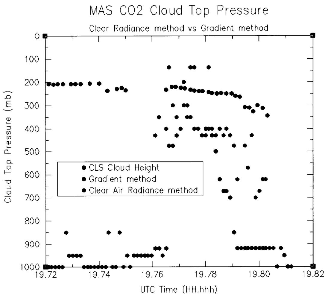
Figure 5. MAS CO<sub>2</sub> cloud top pressure estimates on April 26, 1996 over Kansas. Cloud top pressure from CLS lidar also shown as validation. MAS CO<sub>2</sub> algorithm tracks relative variation of cloud top pressure. Very thin cirrus cloud is unresolved in MAS data before 19.76 UTC.
