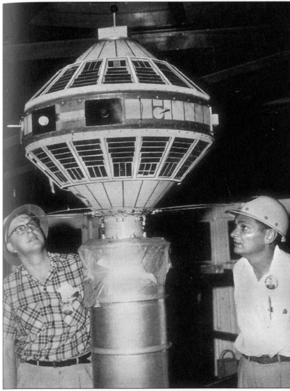
Professor Suomi and Herman La Gow inspect the spinning, polar-orbiting satellite on which the flat plate radiometer flew.
