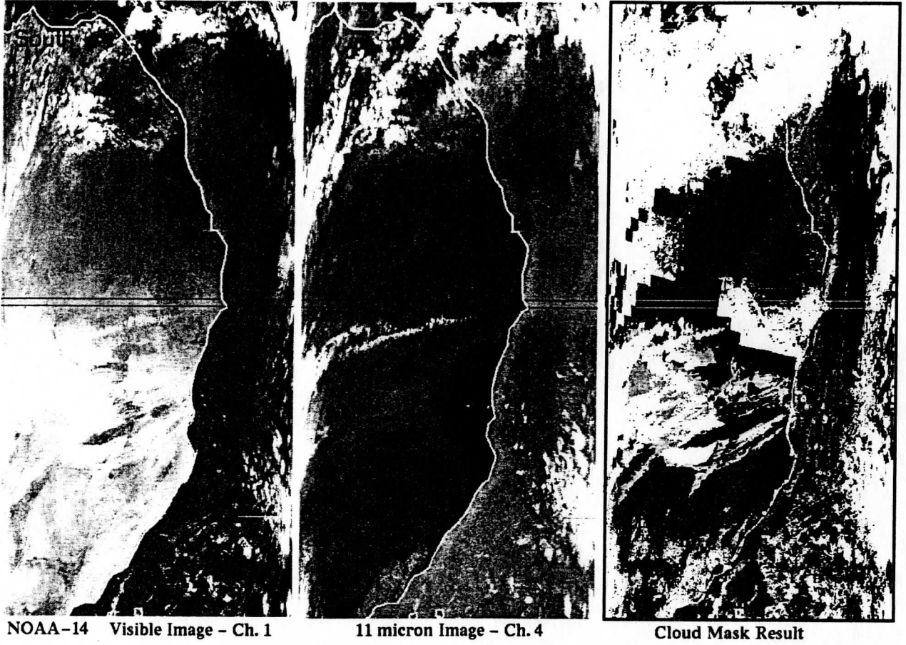
Figure 6. An example cloud mask, together with images at two AVHRR bands, obtained over the eastern Atlantic and west Africa. South is at the top of the figure.
